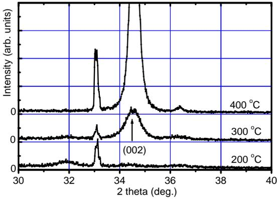
Fig. 1. X-ray diffraction from ZnO films grown at different temperatures. The arrow indicates wurtzite (002) peak position, 34.422°.
