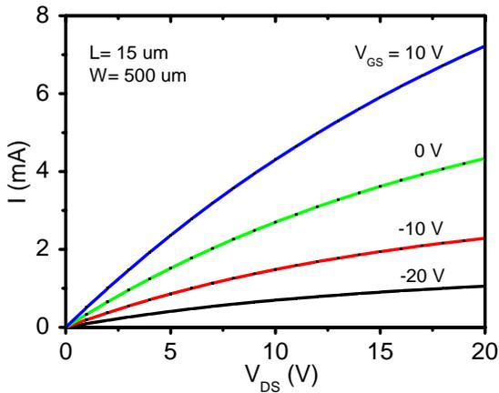
Fig. 2. Current-voltage characteristics of ZnO TFT, grown at 300°C.
