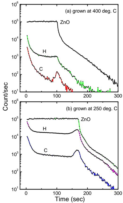
Fig. 4. SIMS profiles of hydrogen and carbon in ZnO.
