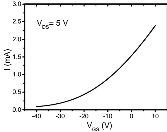
Fig. 3. Current change by gate voltage. The device is the same one used in Fig. 2.
