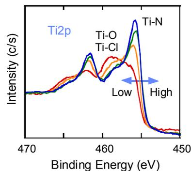
Fig. 3 Ti2p XPS spectra of divided CVD-TiN films. Ti-O and Ti-Cl bonds were shown from low divided number CVD-TiN.
