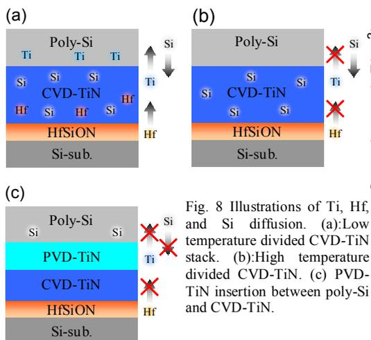
Fig. 8 Illustrations of Ti, Hf, and Si diffusion. (a): Low temperature divided CVD-TiN stack. (b): High temperature divided CVD-TiN. (c) PVD-TiN insertion between poly-Si and CVD-TiN.
