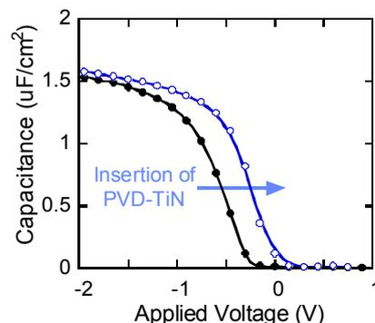
Fig. 10 Effect of insertion of PVD-TiN between poly-Si and CVD-TiN metal gate. With PVD-TiN cap, divided CVD-TiN metal gate still maintain suitable effective work function for p-MISFETs.
