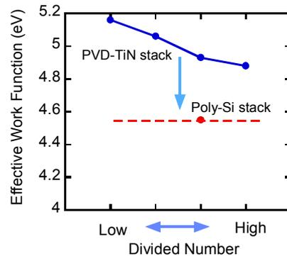
Fig. 6 Effective work function of divided CVD-TiN with PVD-TiN and poly-Si cap. By poly-Si capping, effective work function shifted to 4.6 eV.
