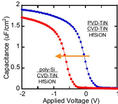
Fig. 5 C-V characteristics of CVD-TiN/HfSiON stacks with PVD-TiN and poly-Si cap layer. CV curve shifted to mid-gap by poly-Si capping.
