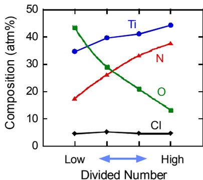
Fig. 4 Influence of divided number in a divided TiN-CVD on film composition obtained from XPS results.
