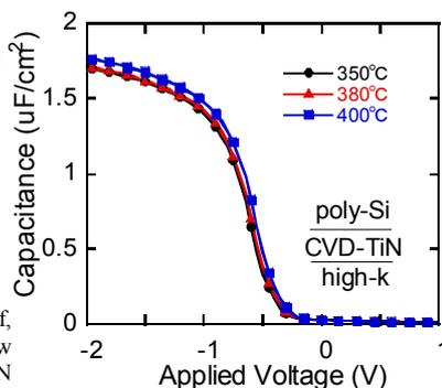
Fig. 9 C-V characteristics of poly-Si/CVD-TiN/HfSiON stacks. CV curves slightly shifted to the positive bias with the CVD-TiN of high temperature deposition.
