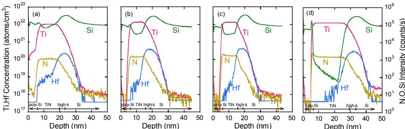
Fig. 7 SIMS depth profiles of poly-Si/CVD-TiN/HfSiON stacks [(a) – (c)], and poly-Si/PVD-TiN/CVD-TiN/HfSiON stack [(d)]. The deposition temperature of divided CVD-TiN are (a) 350°C, (b) 380°C, and (c) 400°C. By increasing the deposition temperature of CVD-TiN, the diffusion of Si, Ti, and Hf tended to decrease. By PVD-TiN capping, Si diffusion completely suppressed.
