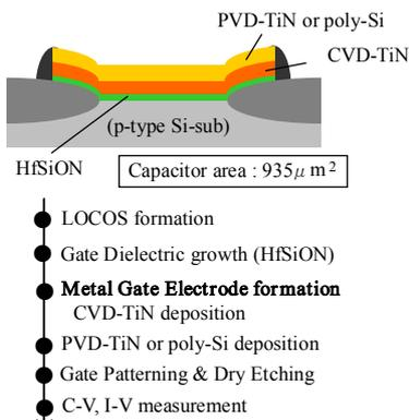
Fig. 1 MIS capacitor structure and its formation flow.
