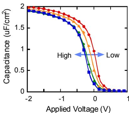
Fig. 2 C-V characteristics of divided CVD-TiN gate stacks by various conditions. Low divided number leads the effective work function high.
