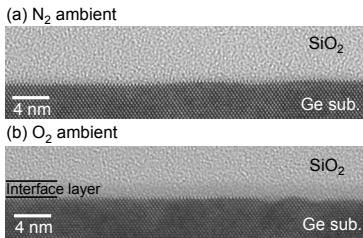
Fig. 1: Cross-sectional TEM images of the samples (a)  $N_2$ , (b)  $O_2$ , respectively.
