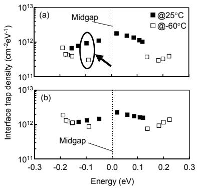
Fig. 6: Interface trap density distributions measured at  $25^\circ\text{C}$  and  $-60^\circ\text{C}$  (a) without including the effect of the surface potential fluctuation and (b) including that.
