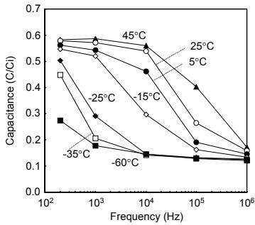
Fig. 3: Dependence of capacitance at midgap voltage on frequency for the sample  $N_2$  at various measurement temperatures.
