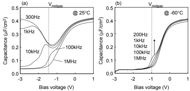
Fig. 2: C-V curves of the sample  $N_2$  measured at various frequencies at (a)  $25^\circ\text{C}$  and (b)  $-60^\circ\text{C}$
