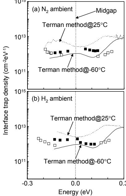
Fig. 4: Comparison of interface trap density distributions measured at  $25^\circ\text{C}$  and  $-60^\circ\text{C}$  of the samples (a)  $N_2$ , (b)  $H_2$ , (c)  $O_2$  and (d)  $NH_3$  by using Terman and the conductance methods, where (■) and (□) indicate results of the conductance method at  $25^\circ\text{C}$  and  $-60^\circ\text{C}$ , respectively.
