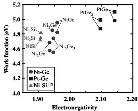
Fig. 7 The dependence of the work function values on the electronegativities for the Ni-Ge, Ni-Si<sup>[2]</sup> and Pt-Ge gate electrodes.
