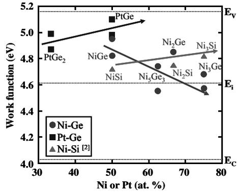
Fig. 6 The metal (Ni, Pt) composition ratio dependence of the work function values for the Ni-Ge, Ni-Si<sup>[2]</sup> and Pt-Ge gate electrodes.
