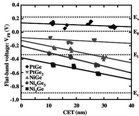
Fig. 5 CET dependence of the flat-band voltages for the MOS capacitors with the NiGe, Ni<sub>5</sub>Ge<sub>3</sub>, Ni<sub>3</sub>Ge, PtGe<sub>2</sub> and PtGe gate electrodes.
