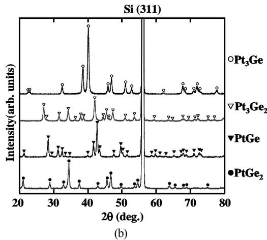
Fig. 1 XRD profiles of (a) Ni/Ge/SiO<sub>2</sub>/Si and (b) Pt/Ge/SiO<sub>2</sub>/Si samples after RTA.
