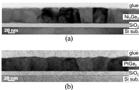
Fig. 2 Cross-sectional TEM images of (a) Ni<sub>5</sub>Ge<sub>3</sub> and (b) PtGe<sub>2</sub> films.
