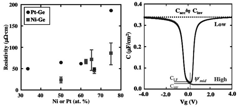
Fig. 3 The metal composition ratio dependence of the resistivities for the Ni-Ge and Pt-Ge films.
