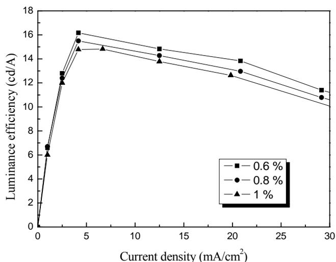
Fig. 3. The luminance efficiency-current density characteristics of the white PHOLEDs.
