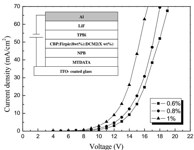
Fig 1. The current density-voltage (J-V) characteristics of the white PHOLEDs. Inset: The device's structure of the white PHOLED studied.
