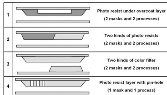
Fig. 1 4 basic and novel-type structures of color filter
