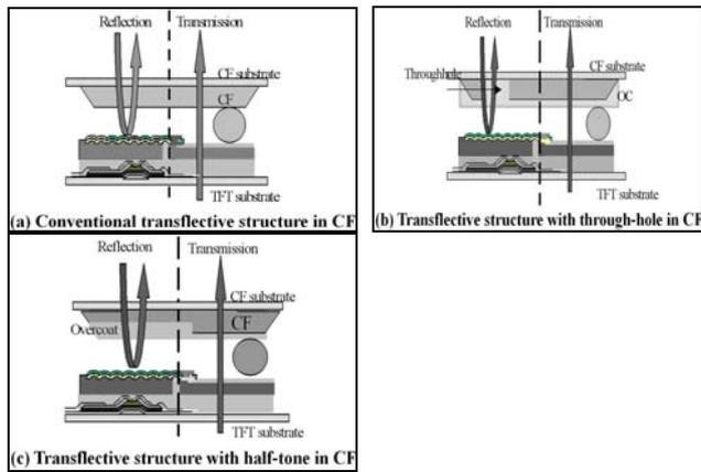
Fig. 2 Transfective structure of LCD cell with color filter type: (a) conventional type, (b) through-hole type and (c) half-tone type
