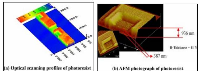
Fig. 3 (a) Optical scanning profiles, (b) atomic force microscopic photographs of through-hole type or half-tone type color filter
