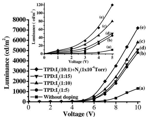
**Fig.1.** The output luminance of OLEDs as a function of driving voltage for split HTL evaporation conditions; curve (a) without doping, curve (b) with weight ratio TPD : $I_2$  =1:5, curve (c) with weight ratio TPD : $I_2$  =1:10, curve (d) with weight ratio TPD : $I_2$  =1:15 and curve (e) with weight ratio TPD : $I_2$  =1:10 under  $N_2$   $1 \times 10^{-4}$  Torr ambient. The inset shows the zoom for the driving voltage 0 to 5V
