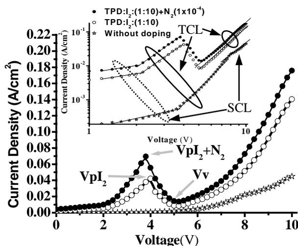
**Fig.4.** The current density-voltage curves with linear and log-log scale (inset) of OLEDs with iodine dopant under nitrogen ambient (TPD/  $I_2$  =1/10 and  $N_2$   $1 \times 10^{-4}$  Torr ambient), the OLEDs with iodine dopant (TPD/  $I_2$  =1/10) and without iodine dopant are included.
