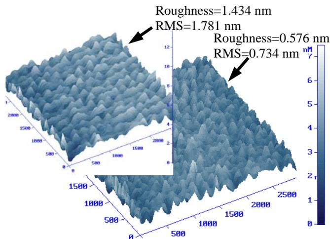
**Fig.3.** AFM micrographs of iodine doped TPD film with  $1 \times 10^{-4}$  Torr nitrogen ambient and without (insert)
