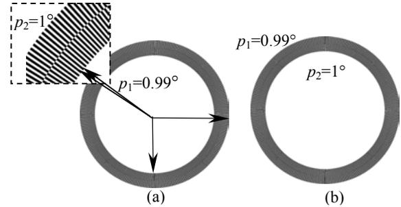
Fig.3 vernier-like duplex radial gratings in the circumference of 4-inch (a) upper and (b) lower wafer
