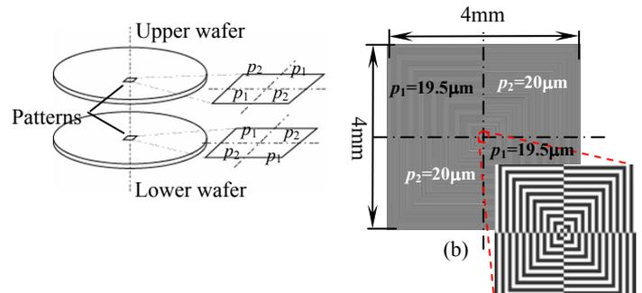
Fig.1 (a) schematic diagram of patterns on two wafers respectively (b) a centro-symmetric pattern of square gratings with line width of  $10\mu\text{m}$  in the center of the wafer
