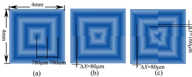
Fig.2 Computer generated moiré fringes produced by superimposing two centro-symmetric patterns of square gratings with different misalignments without rotation; (a) well-matched (b)  $\Delta x=1\mu\text{m}$  (c)  $\Delta x=1\mu\text{m}$ ,  $\Delta y=2\mu\text{m}$
