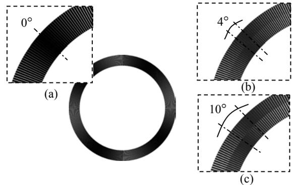
Fig.4 Computer generated moiré fringes produced by superimposing duplex radial gratings in the circumference of two wafers with different misalignments of  $\theta$ -axis; (a) no rotation (b)  $\Delta\theta = 0.02^\circ$  (c)  $\Delta\theta = 0.05^\circ$
