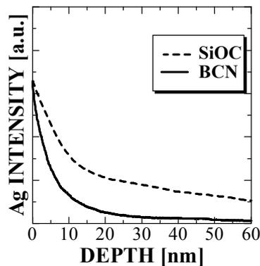
Fig.5. The depth profiles of Ag in BCN and SiOC dielectric films after annealing.
