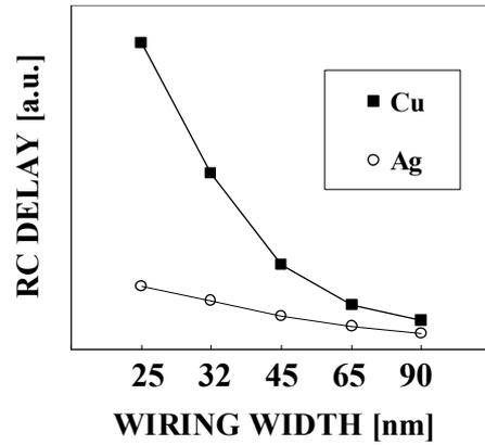
Fig. 2 The simulation result using Ag and Cu with various wiring widths. Simulation Condition: Diffusion barrier width 20nm for (Cu) and 5nm for (Ag). Barrier metal from 90nm generation, every generation reduces 15%.
