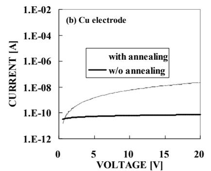
Fig.4. The I-V characteristics before and after annealing when electrodes were (a) Ag and (b) Cu electrode, respectively.
