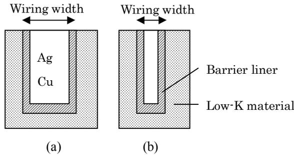
Fig. 1. The model of interconnection how to change from (a) 90 nm to (b) below 50 nm for the future high-density circuit.
