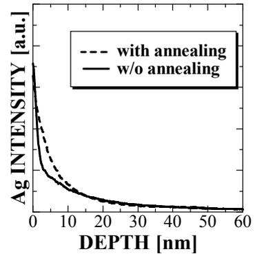
Fig. 6. The depth profiles of Ag in BCN film before and after annealing.
