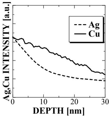
Fig.3. Ag and Cu depth profile in SiOC film after annealing.
