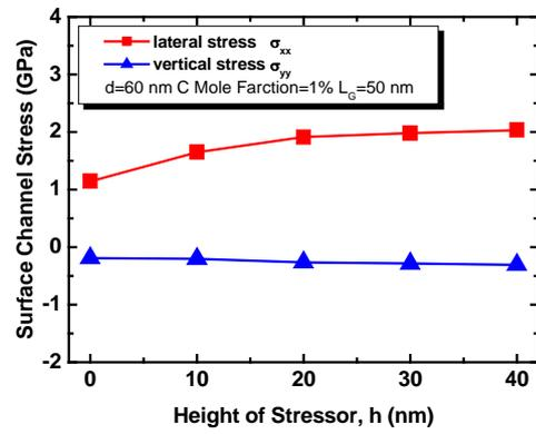
Fig. 2 Raising the stressor height  $h$  leads to more tensile lateral stress  $\sigma_{xx}$ .
