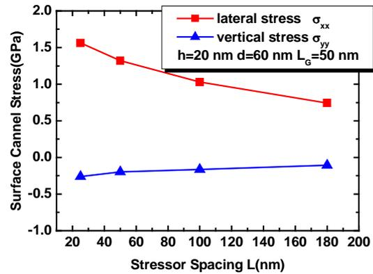
Fig. 5 Lateral and vertical strain components,  $\sigma_{xx}$  and  $\sigma_{yy}$ , respectively, in the surface channel plotted as a function of the spacing between the source stressor and drain stressor.
