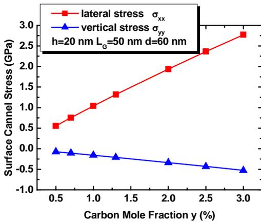
Fig. 4 Lateral and vertical strain components,  $\sigma_{xx}$  and  $\sigma_{yy}$ , respectively, in the surface channel plotted as a function of the C mole fraction  $y$  in the  $\text{Si}_{1-y}\text{C}_y$  stressor.
