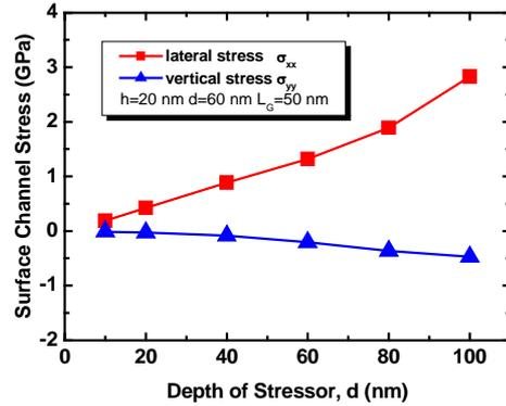
Fig. 3 Lateral and vertical strain components,  $\sigma_{xx}$  and  $\sigma_{yy}$ , respectively, in the surface channel plotted as a function of the depth of the  $\text{Si}_{1-y}\text{C}_y$  stressor.
