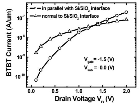
Fig.9 BTBT currents in parallel with Si/SiO<sub>2</sub> interface and normal to Si/SiO<sub>2</sub> interface as a function of drain voltage.
