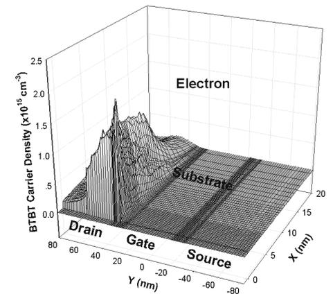
Fig.6 BTBT electron density distribution in a 45-nm channel-length Si nMOSFET.
