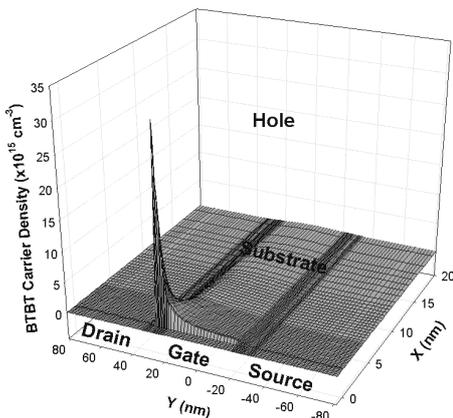
Fig.7 BTBT hole density distribution in a 45-nm channel-length Si nMOSFET.
