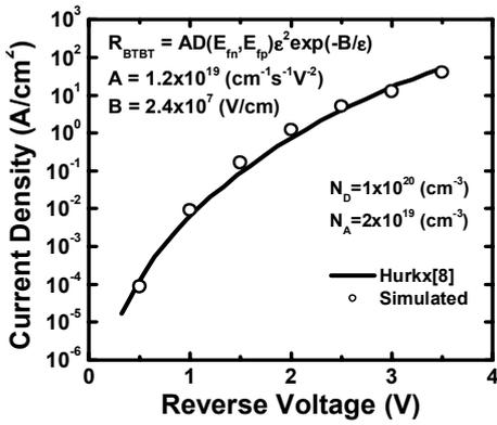
Fig.4 Simulated current density as a function of reverse voltage. For comparison, the measurement results [8] are also shown.
