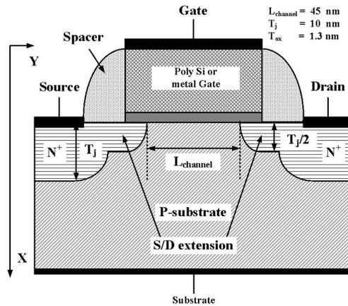
Fig.5 Schematic of a 45-nm channel-length Si nMOSFET with S/D extension.
