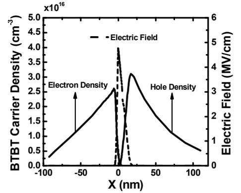
Fig.3 Band-to-band tunneling carrier density and electric field in a PN junction.
