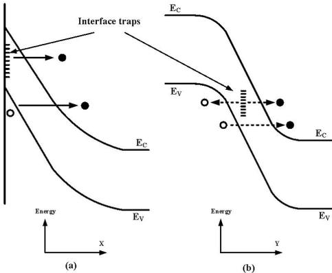
Fig.1 BTBT mechanisms including band-trap-band tunneling in nMOSFETs under deep depletion: (a) normal to Si/SiO<sub>2</sub> interface (b) in parallel with Si/SiO<sub>2</sub> interface.
