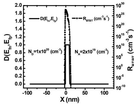
Fig.2 Net-rate factor  $D(E_{fm}, E_{fp})$  and band-to-band tunneling rate in a PN junction.
