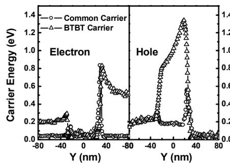
Fig.8 BTBT carrier average energy distribution along the channel near the Si/SiO<sub>2</sub> interface.
