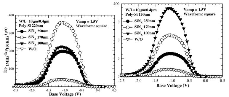
Fig. 5 ( $I_{CP,1MHz} - I_{CP,100K}$ ) of devices for different SiN capping layers versus base voltage ( $W/L=10\mu\text{m} / 0.4\mu\text{m}$ ) (a) 220nm (b) 150nm poly-Si gate. The ( $I_{CP,1MHz} - I_{CP,100K}$ ) is for the purpose of leakage current correction
