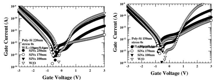
Fig.9  $I_g$  versus gate voltage. the split w/o SiN capping layer depicts the largest substrate injection current among all splits. The splits with 170nm SiN capping layer, 150nm and 220nm poly-Si gate, show the lowest substrate injection current. (a) 220nm (b) 150nm poly-Si gate
