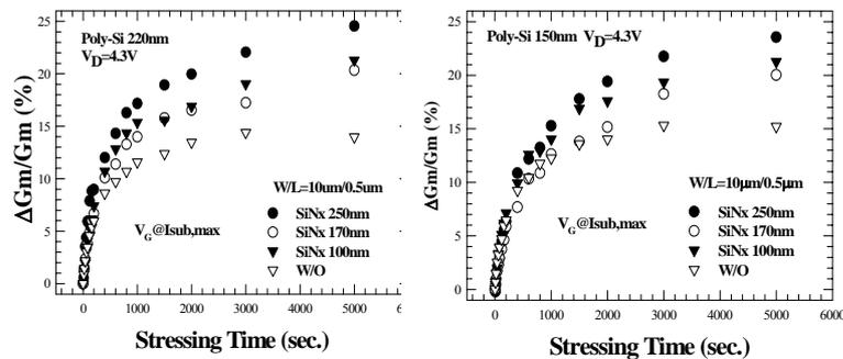
Fig. 8 Stressing time dependence of  $G_m$  degradations. Devices are stressed at  $V_D=4.3V$ , and  $V_G$  is at  $I_{SUB,max}$  at  $V_D=4.3V$ . (a)220nm (b) 150nm poly-Si gate
