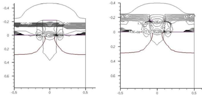
Fig.4 Simulation stress distribution along the channel of the splits with 250nm SiN layer. (a) 220nm (b) 150nm poly-Si gate.
