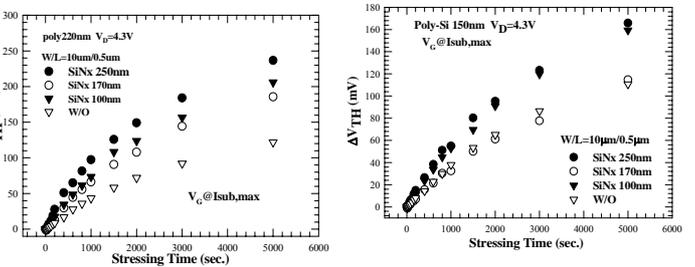
Fig. 7 Stressing time dependence of  $V_{TH}$  degradations. Devices are stressed at  $V_D=4.3V$ , and  $V_G$  is at  $I_{SUB,max}$  at  $V_D=4.3V$ . (a)220nm (b)
