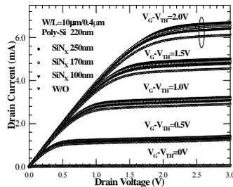
Fig. 2  $I_D$  versus  $V_D$  for nMOSFET ( $W/L=10\mu\text{m} / 0.4\mu\text{m}$ ) 220nm poly-Si gate
