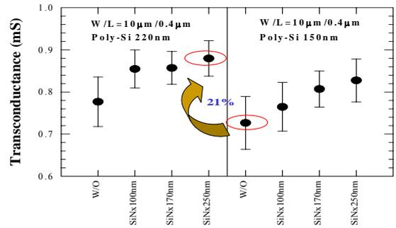
Fig.3  $G_m$ , each point was obtained from 10 devices, versus the splits of different SiN capping layer ( $W/L=10\mu\text{m} / 0.4\mu\text{m}$ ).
