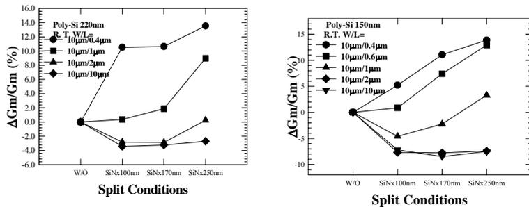
Fig.6  $G_m$  for nMOSFETs of different gate length at room temperature versus different SiN capping layers. (a) 220nm (b) 150nm poly-Si gate. Each point was obtained from 10 devices
