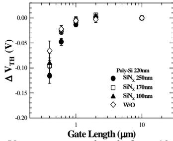
Fig.1  $V_{TH}$  versus gate length from  $10\mu\text{m}$  down to  $0.4\mu\text{m}$ . Every error estimation point is from ten devices 220nm poly-Si gate
