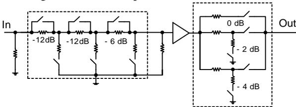
Fig. 6. The circuits of feedback variable attenuator
