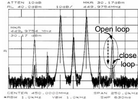
Fig. 8. Characteristic of CFL transmitter (@450MHz)
