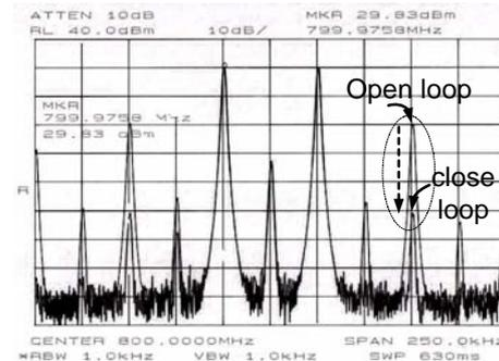
Fig. 9. Characteristic of CFL transmitter (@800MHz)
