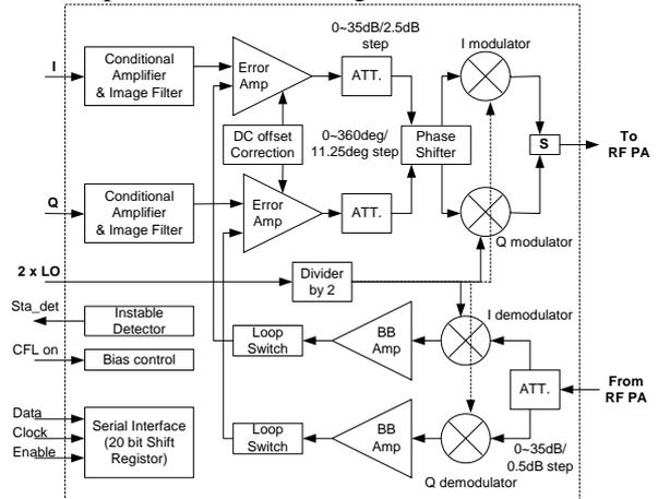
Fig.2. Block diagram of CFL chip
