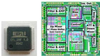
Fig. 7. The implemented Cartesian feedback loop chip
