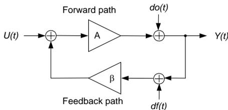
Fig.1. The Equivalent model of CFL Transmitter.
