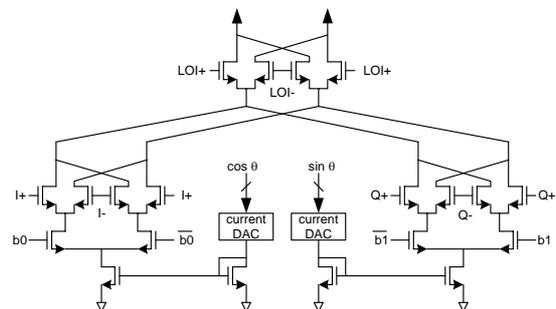
Fig. 3. The circuit of phase shifter
