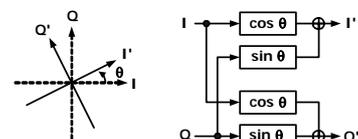
Fig. 4. Concept of phase shifting
