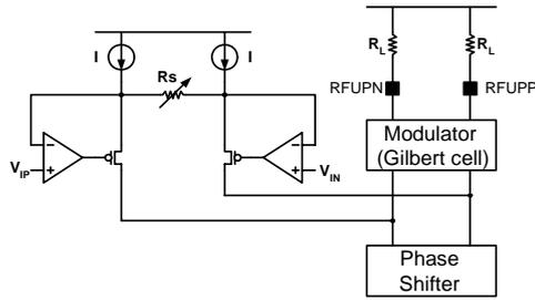
Fig. 5. The circuits of I/Q modulator for gain control
