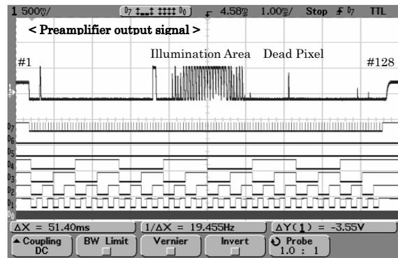
Fig. 6. Preamplifier output waveform(top waveform) and control signals of 1 by 128 detector array under the IR laser illumination
