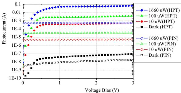
Fig. 4. DC optical properties of HPT and P-i-N photodetector with the same light absorbing area at different incident optical powers
