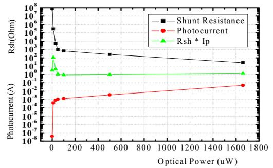
Fig. 5. Relationship between photocurrent level and shunt resistance under different incident power
