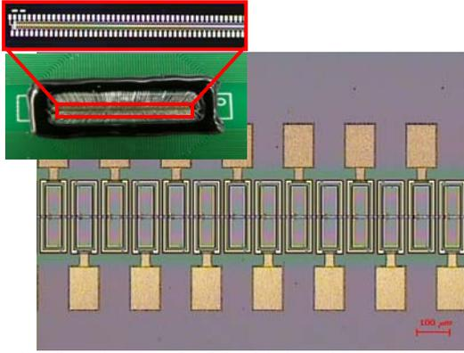
Fig. 3. Microphotograph of the fabricated HPT 1 by 128 array
