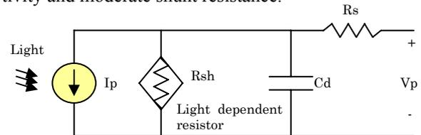
Fig. 1. Equivalent model of HPTs
