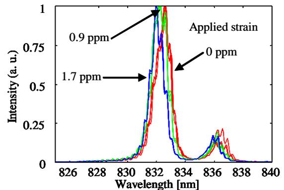
Fig. 5 Change of a radiation spectrum of a laser chip under an applied uni-axial strain
