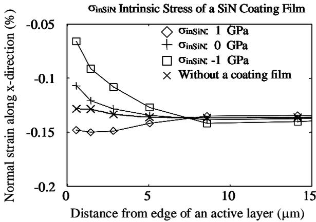
Fig. 3 Change of a strain distribution in an active layer of a laser chip due to the intrinsic stress of a mirror film
