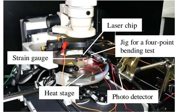
Fig. 4 Measurement of a radiation spectrum of a laser chip under a four-point bending test
