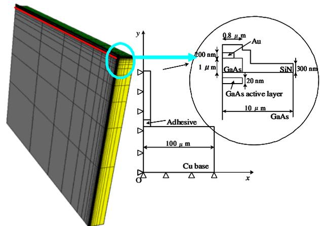
Fig. 1 Finite element analysis model of a laser chip.
