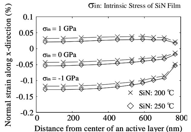
Fig. 2 Change of a strain distribution in an active layer of a laser chip due to the intrinsic stress of a Si<sub>3</sub>N<sub>4</sub> film
