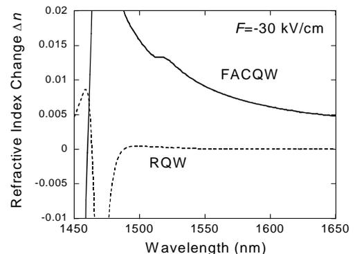
Fig.2 Electrorefractive index change  $\Delta n$  (for TE mode) of the InGaAs/InAlAs FACQW and RQW (6.5nm).
