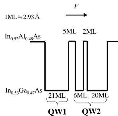
Fig.1 Schematic diagram of InGaAs/InAlAs FACQW for 1.55  $\mu\text{m}$  wavelength.
