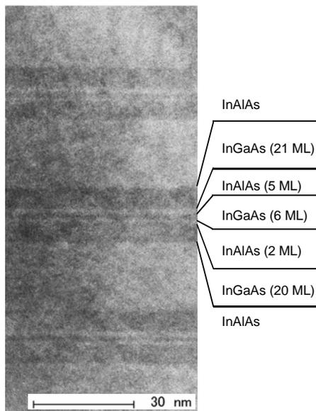
Fig.3 Transmission electron microscopy (TEM) image of the cross-section of a multiple InGaAs/InAlAs FACQW sample.
