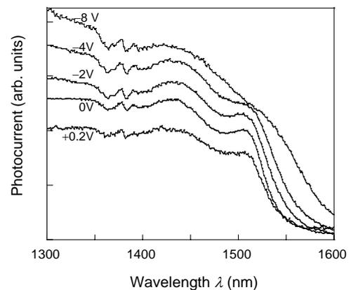
Fig.5 Measured photoabsorption current spectra of the grown multiple InGaAs/InAlAs FACQW.
