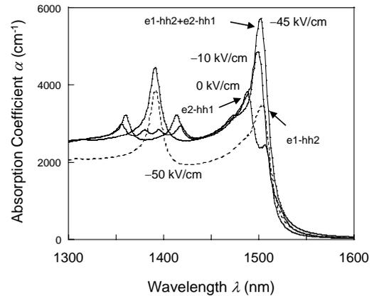
Fig.4 Calculated absorption coefficient spectra of InGaAs/InAlAs FACQW.
