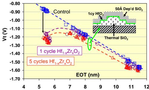
Fig. 4  $V_t$ -EOT behavior for cake oxide/ $60\text{\AA}$   $SiO_2$  versus cake oxide/1-5cy  $HfO_2$ / $60\text{\AA}$   $SiO_2$ .
