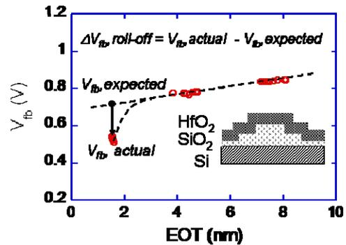
Fig. 1  $\Delta V_{\text{fb}}$  roll-off behavior and picture of cake oxide formation.
