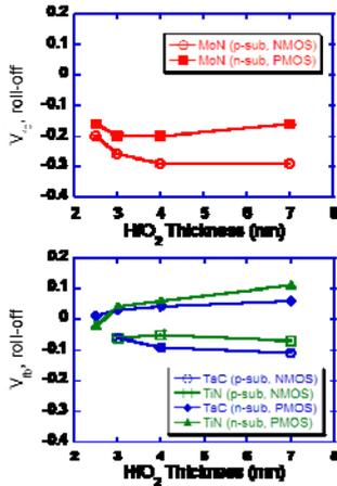
Fig. 3 Magnitude of  $\Delta V_{fb}$  roll-off (V) for  $Mo_2N$  (top) and TiN, TaC (bottom) for different  $HfO_2$  thickness
