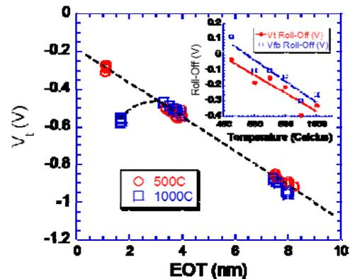
Fig. 2  $V_t$ -EOT comparison for 500°C & 1000°C anneal and magnitude of the  $\Delta V_{\text{fb}}$  roll-off 500°C-1000°C (inset).
