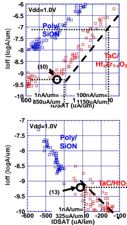
Fig. 5 Ion-Ioff plots for TaC nFET and TaC buried channel pFET
