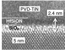
Fig. 5 Cross-sectional TEM image of TiN/HfSiON/SiO<sub>2</sub>/Si stacks.
