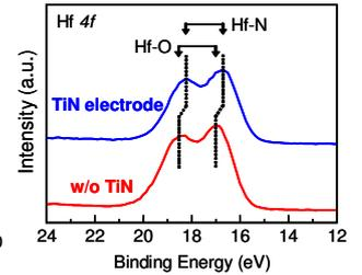
Fig. 7 XPS analysis of Hf-silicates; (a) as-fabricated HF-silicate surface, (b) after TiN growth (TiN overlayer was removed by wet etching).
