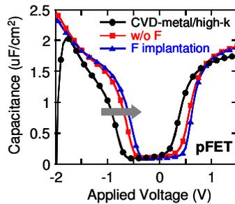
Fig. 12 Effects of PVD-based in-situ fabrication method and F implantation on V<sub>th</sub> tuning.
