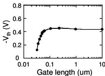
Fig. 14 V<sub>th</sub> roll-off characteristics of pMISFET with poly-Si/TiN/HfSiON gate stacks.
