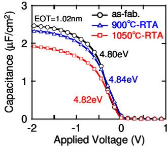
Fig. 4 C-V curves of metal/high-k capacitors fabricated with PVD-based in-situ fabrication method before and after RTA (900, 1050°C).
