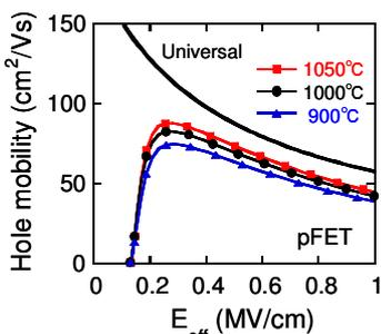
Fig. 11 Dependence of hole mobility of gate-first metal/high-k pMISFETs on RTA conditions.
