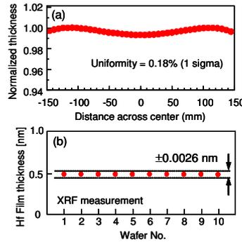
Fig. 2 Basic performance of PVD system; (a) film uniformity, (b) reliability of Hf ultrathin film.
