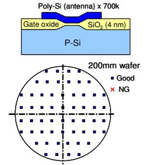
Fig. 3 Damage characterization using antenna MOS capacitors. Antenna ratio was 700k.
