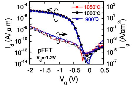
Fig. 10 Dependence of Id-Vg and Ig-Vg curves of pFETs on RTA conditions.
