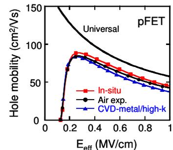
Fig. 13 Change in hole mobility of gate-first pFETs depending on fabrication method of HfSiON dielectrics and TiN electrodes.
