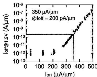
Fig. 15 Ion-Ioff characteristics of pMISFET with poly-Si/TiN/HfSiON gate stacks.
