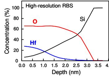
Fig. 6 Depth profile of HfSiON gate dielectric fabricated with in-situ SPIR.
