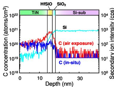
Fig. 8 SIMS profiles of carbon impurity of TiN/HfSiON/SiO<sub>2</sub> stacks.
