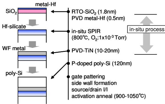
Fig. 1 Concept and fabrication flow of poly-Si/TiN/HfSiON gate stacks with PVD-based in-situ SPIR method.
