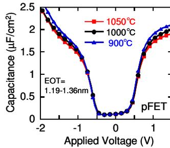
Fig. 9 Dependence of C-V curves of gate-first pFETs on RTA conditions.
