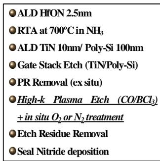
Fig 1. Gate stack process flow of MOSFET with TiN/HfON gate stack, high-k film is removed by plasma etch and treated with in situ O<sub>2</sub> or N<sub>2</sub> plasma
