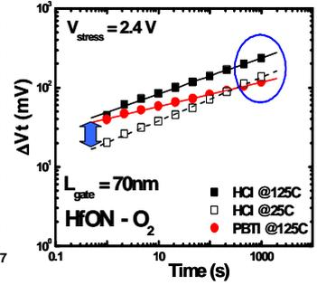
Fig 10. Comparison of V<sub>th</sub> shift between HCl @25°C, HCl @125°C, and PBTI @125°C. For short channel devices, high temperature HCl degradation needs to be treated as a key reliability criterion.
