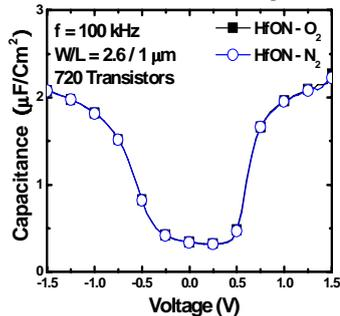
Fig 3. The CV curves of the perimeter-intensive array transistor in HfON with either an O<sub>2</sub> or N<sub>2</sub> plasma treatments; The capacitance of both cases seems to be the same.
