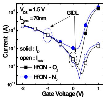
Fig 4. GIDL characteristics in HfON with O<sub>2</sub> or N<sub>2</sub> treatment; The GIDLs for both HfON devices show similar slopes. But, the GIDL-dominated point of the O<sub>2</sub>-treated sample is lower than that of the N<sub>2</sub>-treated sample
