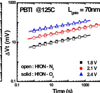
Fig 5. Comparison of V<sub>th</sub> shifts induced by PBTI; PBTI of both O<sub>2</sub>- and N<sub>2</sub>-treated devices showed similar V<sub>th</sub> degradation, indicating that PBTI is not correlated with the gate edge profile.
