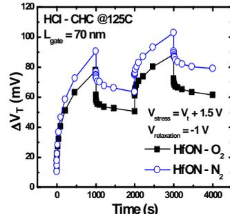
Fig 12. Comparison of V<sub>th</sub> shift under V<sub>stress</sub> = V<sub>th</sub> + 1.5V and V<sub>relaxation</sub> = -1V in HfON with O<sub>2</sub> or N<sub>2</sub> treatment; the O<sub>2</sub>-treated sample showed less V<sub>th</sub> degradation and a higher recovery rate.
