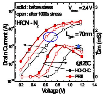
Fig 11. Comparison of drain current and G<sub>m</sub> under V<sub>stress</sub> = 2.4V after PBTI or HCl at 125°C; HCl characteristics showed more significant drain current and G<sub>m</sub> degradation.
