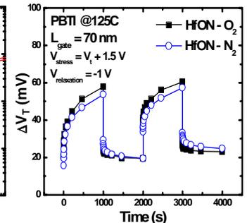
Fig 6. V<sub>th</sub> recovery rate under V<sub>stress</sub> = V<sub>th</sub> + 1.5V, and V<sub>relaxation</sub> = -1V; Similar recovery rate regardless of O<sub>2</sub> and N<sub>2</sub> treatment, indicating that PBTI is not correlated with the gate edge profile.
