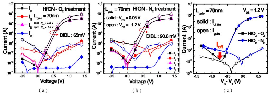
Fig 2. Transistor current-voltage (I-V) characteristics with (a) O<sub>2</sub> treatment and (b) N<sub>2</sub> treatment, and (c) normalized drain and gate current; HfON O<sub>2</sub>-treated samples show a 20X lower off-state leakage current and slightly lower DIBL compared to N<sub>2</sub> treated samples.
