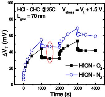
Fig 7. Comparison of V<sub>th</sub> shift induced by HCl; O<sub>2</sub> treated sample showed not only smaller V<sub>th</sub> degradation and but also higher recovery rate compared to N<sub>2</sub> treated sample.
