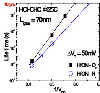
Fig 9. Comparison of HC lifetime between O<sub>2</sub> and N<sub>2</sub> plasma treated devices at 25°C. Excellent lifetime can be obtained by O<sub>2</sub> treated devices compared to N<sub>2</sub> treated devices.
