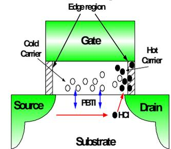
Fig 8. Schematic diagram of charge behavior during stress; Heterogeneous leakage path in the gate edge region creates deeper traps during HCl stress.
