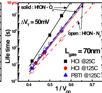
Fig 13. Lifetime comparison between HCl and PBTI, and O<sub>2</sub> and N<sub>2</sub> treatment. The devices with O<sub>2</sub> plasma treatment shows larger calculated device life time.
