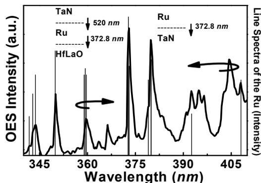
Fig. 6 Optical Emission Spectra (OES) intensities detected during etching of Ru gate stack in  $\text{O}_2$  plasma, line spectra of the Ru elements also shown on the right axis. The endpoint of TaN, etched in  $\text{Cl}_2$  plasma is obtained using  $520\text{ nm}$  wavelength. When Ru is exposed to  $\text{Cl}_2$  plasma, Ru film is not etched due to formation of nonvolatile  $\text{RuCl}_x$ . Moreover, when HfLaO film is exposed to  $\text{O}_2$  plasma, the high- $k$  film is not etched.
