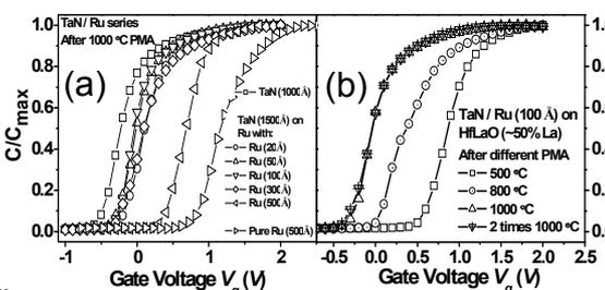
Fig. 2(a) CV curves for TaN/Ru series with different Ru thicknesses after high temperature annealing and (b) TaN/Ru with  $100\text{\AA}$  Ru after different temperature RTA.
