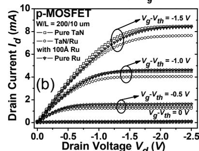
Fig. 3(a) Transfer characteristics of pMOSFETs with TaN/Ru gate stacks. Different Ru thicknesses introduce  $\sim 1.3\text{ V}$   $V_{fb}$  shift; (b) Output characteristics of pMOSFETs with pure TaN, TaN/Ru stack with  $100\text{\AA}$  Ru and pure Ru metal gate after  $1000^\circ\text{C}$  annealing.
