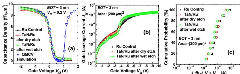
Fig. 9 Comparison of  $C-V$  characteristic (a),  $J_g-V_g$  characteristic (b) and  $J_g$  distribution @  $V_{fb} = -1\text{ V}$  among the Ru control devices and re-deposited Ru layer after removal of TaN layer by dry etch and wet etch respectively.
