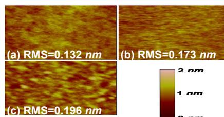
Fig. 7 AFM pictures for pure Ru film (a), TaN/Ru stacks after TaN etching in both dry and wet mode, respectively (b) & (c).  $0.064\text{ nm}$  variation of RMS indicates negligible physical damage to the original Ru layer during the etch processes.
