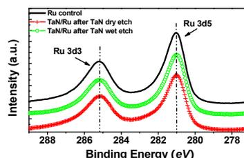
Fig. 8 XPS spectra of Ru 3d taken from pure Ru film, TaN/Ru stacks after TaN etching in both dry and wet mode. The consistent spectra indicate minimal TaN residue after etch process and no significant influence on chemical bond change for the originally underlying Ru layer.
