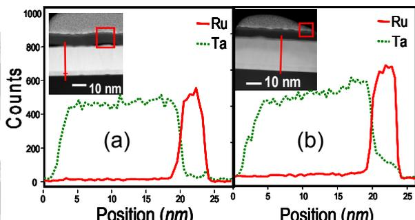
Fig. 4 EDX analysis for TaN and Ru stack, (a) As deposited and (b) After  $1000^\circ\text{C}$  5 sec RTA. Obvious Ta diffusion into Ru layer up to the interface between Ru and HfLaO was observed after high temperature annealing.
