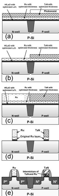
Fig. 5(a)-(e) Schematic illustration of the process flow for possible dual metal gate CMOS integration.
