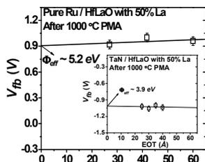
Fig. 1  $V_{fb}$  as a function of EOT for pure Ru and HfLaO with  $\sim 50\%$  La stacks after  $1000^\circ\text{C}$  annealing. The inset shows the case of TaN/HfLaO stacks.
