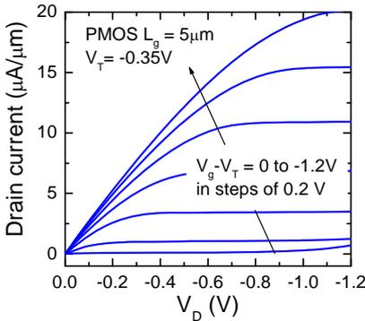
**Fig. 7** I<sub>d</sub>-V<sub>d</sub> characteristics for tensile strained Ge p-MOSFET.
