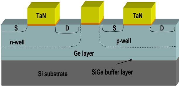
**Fig. 1** Schematic diagram of the Ge MOSFET fabricated on Si wafer. Gate stack consists of 6nm HfO<sub>2</sub>/TaN (100nm).
