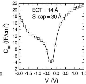
**Fig. 5** C-V characteristics for Ge p-MOSFET. HfO<sub>2</sub>(6nm)/TaN on Si/Ge shows accumulation EOT of 14 Å.
