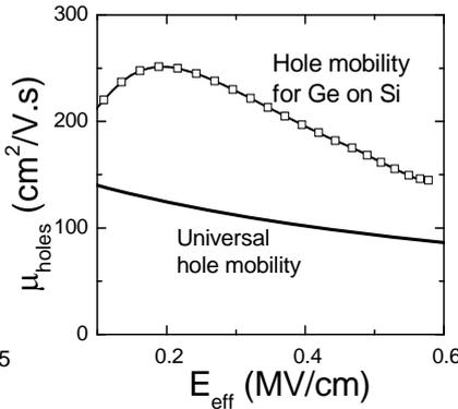
**Fig. 11** Hole mobility for Ge p-MOSFET measured using split CV method. 2X hole mobility improvement is achieved as compared to Si universal mobility .
