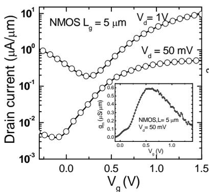
**Fig. 10** I<sub>d</sub>-V<sub>g</sub> characteristics for strained Si/Ge channel n-MOSFET. The insert shows the g<sub>m</sub> for V<sub>DS</sub> = 50 mV.
