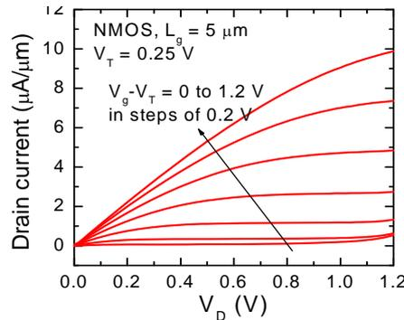
**Fig. 8** I<sub>d</sub>-V<sub>d</sub> characteristics for s-Si/Ge n-MOSFET on n-Si bulk.
