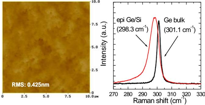
**Fig. 3** AFM of grown Ge surface on 10μm × 10μm pad. Ge surface shows very good surface roughness of RMS of 4.25Å
