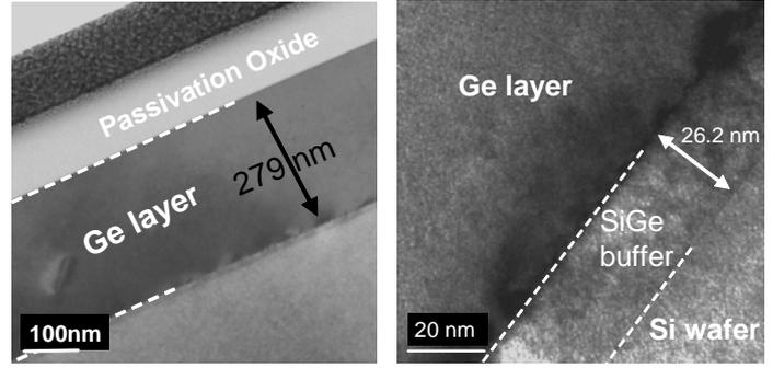
**Fig. 2** HR-TEM images of the heterostructure epitaxial layers of Si/SiGe/Ge layers. Misfit dislocations are confined within the SiGe buffer and at the interface of SiGe/Ge .
