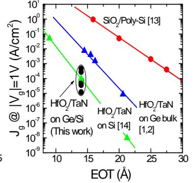
**Fig. 6** High-k gate dielectric leakage current @ |V<sub>g</sub>|=1V as function of EOT. J<sub>g</sub> is comparable to [14] on Si substrate but better than those on Ge bulk [1,2]
