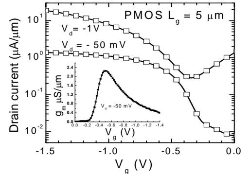
**Fig. 9** I<sub>d</sub>-V<sub>g</sub> characteristics for Ge p-MOSFET. The insert shows corresponding g<sub>m</sub> for V<sub>DS</sub> = -50 mV. High off state leakage is due to lack of halo implant
