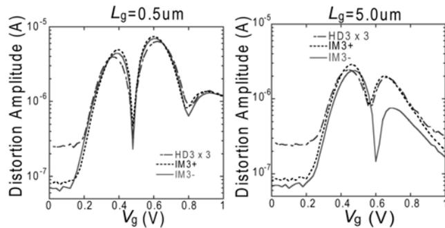
Fig. 5: Comparison of measured distortions for two gate Lengths.
