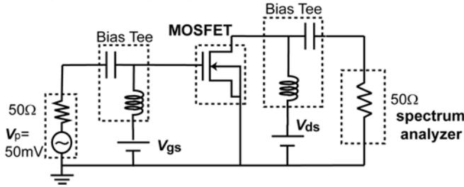
Fig. 4: Circuit used for measuring distortions.
