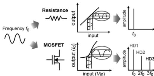
Fig. 1: Origin of harmonic distortions.
