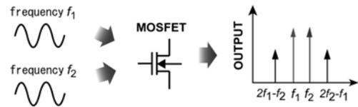
Fig. 2: Origin of inter-modulation (IM) distortions.
