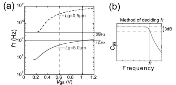
Fig.6: (a) Extracted cut-off frequency  $f_T$  for two gate length;  $L_g=0.5\mu\text{m}$  (dotted line) and  $L_g=5.0\mu\text{m}$  (solid line). The horizontal line with 3GHz is applied for HD3 and IM3+ measurements, and that with 1GHz is applied for IM3- measurements.
