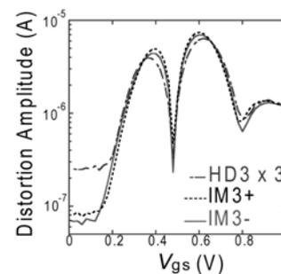
Fig.3: Comparison of measure a distortions for  $L_g/W_g=0.5\mu\text{m}/50\mu\text{m}$ . The measurement conditions, center frequency=1GHz, tone spacing=10MHz, signal amplitude=50mV
