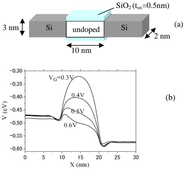
Fig. 2 (a)3D Double Gate MOSFET; (b) The potential profile along the current direction for  $V_{SD}=0.1$  V and  $V_G=0.3-0.6$  V.
