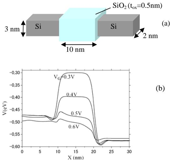
Fig. 3 (a)3D Gate-All-Around MOSFET; (b) The potential profile along the current direction for  $V_{SD}=0.1$  V and  $V_G=0.3-0.6$  V.
