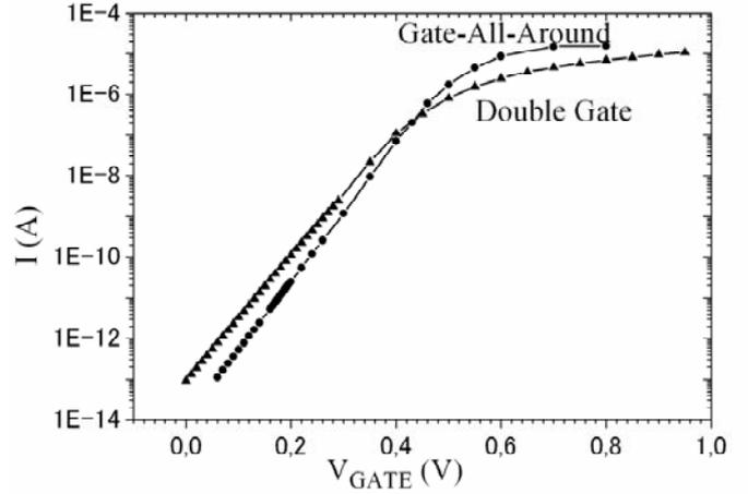
Fig. 4 Drain current in 3D Double Gate and Gate-all-Around MOSFETs as a function of the gate voltage. The applied bias is 0.1 V.
