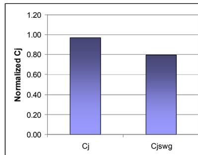
Fig. 8: Normalized  $p^+/NW$  area & sidewall junction capacitance with eSiGe
