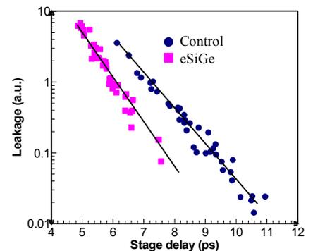
Fig.9: Ring oscillator stage delay vs. leakage current is reduced by ~25% with eSiGe
