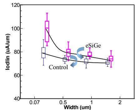
Fig.6: PFET linear current at fixed gate overdrive as a function of device width.
