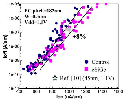
Fig 7: nFET performance enhanced by ~8% using eSiGe process flow.
