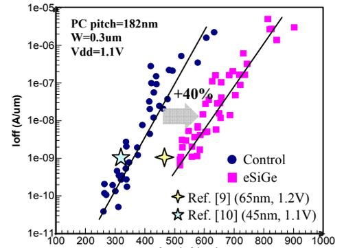
Fig 3: PFET performance improved by ~40% with eSiGe at Vdd=1.1V
