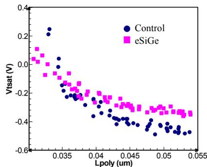
Fig 5: PFET  $V_{tsat}$  as a function of gate length showing improved rolloff performance.
