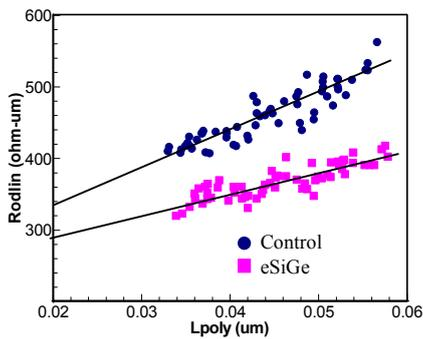
Fig. 4: PFET  $R_{ON}$  at fixed gate overdrive as a function of gate length showing short channel hole mobility enhancement with eSiGe.
