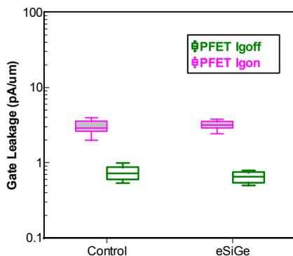
Fig. 10: Comparable pFET gate leakage obtained with eSiGe process
