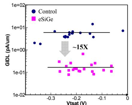
Fig. 12: PFET GIDL current as a function of  $V_{tsat}$ . 15X improvement obtained by eSiGe & implant optimization.
