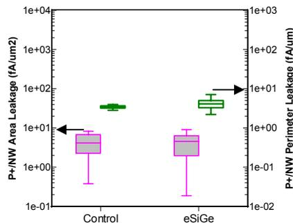
Fig. 11: Area & perimeter junction leakage as a function of process showing comparable performance
