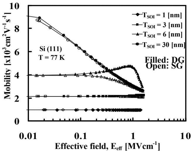
Fig. 3.  $E_{eff}$  dependencies of phonon-limited electron mobility on the (111) Si surface at 77 K as a parameter of  $T_{SOI}$ .
