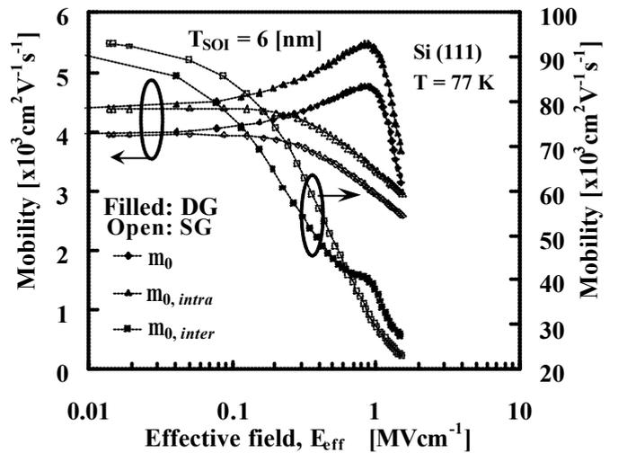
Fig. 5.  $E_{eff}$  dependencies of lowest-subband phonon-limited electron mobility are shown. Acoustic-phonon-scattering-limited mobility,  $m_{0,intra}$ , and optical-phonon-scattering-limited mobility,  $m_{0,inter}$ , are shown separately for SG and DG SOI MOSFET with (111) Si surface channel;  $m_0$  is overall mobility including  $m_{0,intra}$  and  $m_{0,inter}$ .
