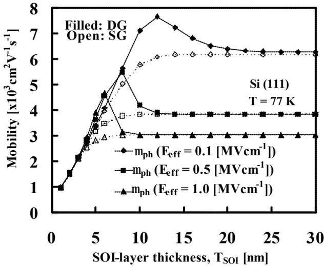
Fig. 2.  $T_{SOI}$  dependencies of phonon-limited electron mobility on the (111) Si surface at 77 K as a parameter of  $E_{eff}$ .
