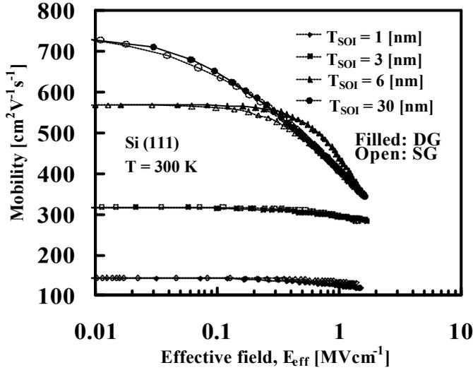
Fig. 1.  $E_{eff}$  dependencies of phonon-limited electron mobility on the (111) Si surface at 300 K as a parameter of  $T_{SOI}$ .
