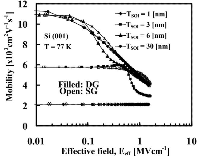
Fig. 4.  $E_{eff}$  dependencies of phonon-limited electron mobility on the (001) Si surface at 77 K as a parameter of  $T_{SOI}$ .
