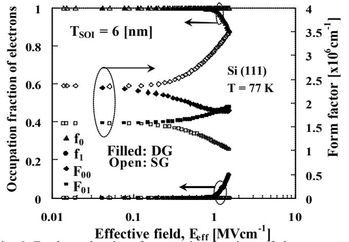
Fig. 6.  $E_{eff}$  dependencies of occupation fractions of electrons sharing the lowest subband for 6-nm- $T_{SOI}$  SG and DG FET's. Respective form factors are also shown for comparison at 77 K.
