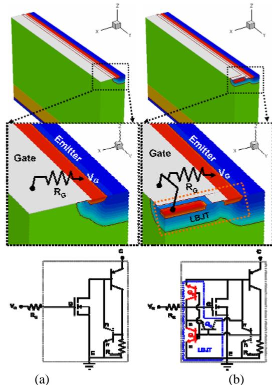
Fig. 1 Device structure and equivalent circuit of the conventional IGBT (a) and the proposed self-protected IGBT (b)
