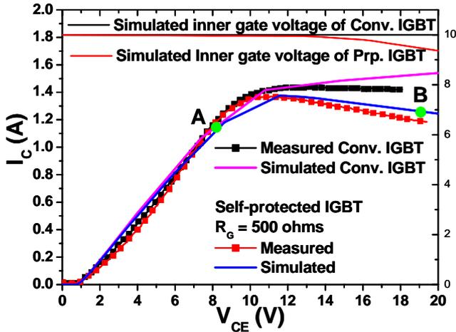
Fig. 2 The measured forward-IV characteristics of the conventional IGBT and proposed IGBT (Point A and B according to  $V_{CE}$ )
