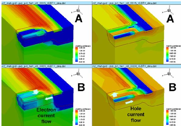
Fig. 3 Electron and hole current distribution in the LBJT according to various  $V_{CE}$  shown in Fig. 2
