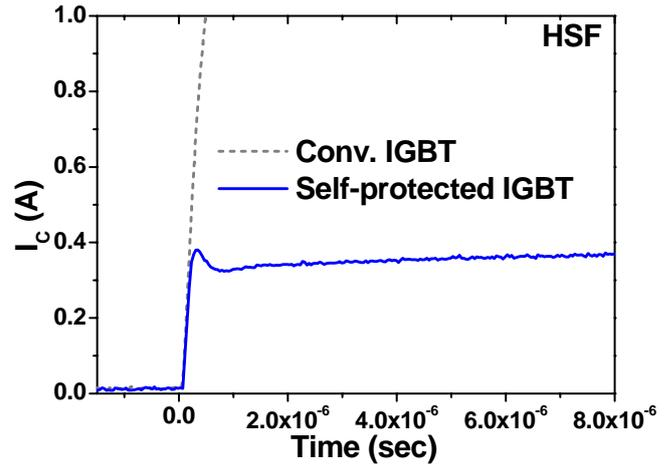
Fig. 4 The measured short-circuit behavior under the hard switching fault condition
