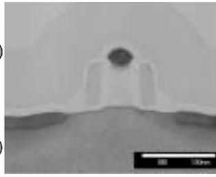
Fig. 3 TEM image of 34 nm NMOS with ALD-SiN spacer
