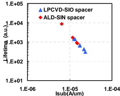
Fig. 11 HCI of 180 nm gate length of NMOS for ALD-SiN and LPCVD-SiO spacer (I/O Transistor)
