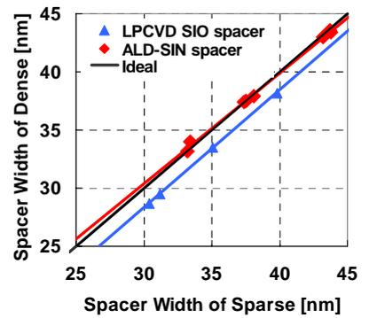
Fig. 9 SEM measurement value of width for sparse and dense pitch
