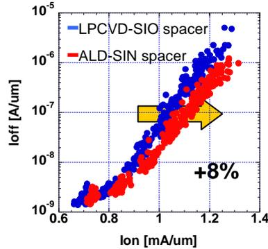
Fig. 6  $I_{on}$  vs.  $I_{off}$  characteristics of at  $V_{dd}=1.0V$
