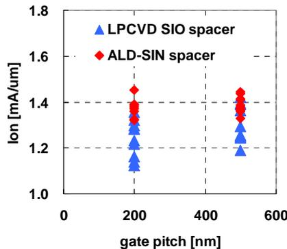
Fig. 8  $I_{on}$  of gate pitch dependency of dense for NMOS
