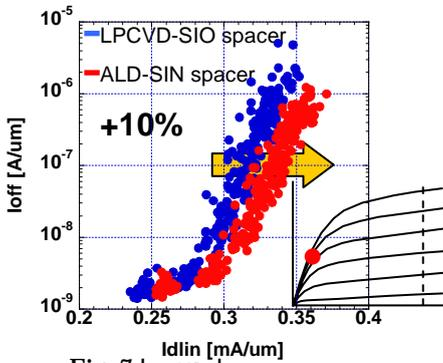
Fig. 7  $I_{dlin}$  vs.  $I_{off}$  characteristics at  $V_{dd}=0.1V$
