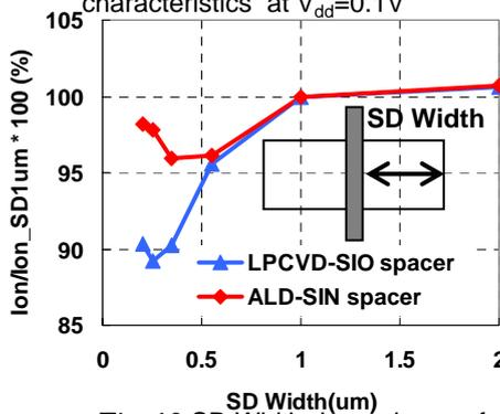
Fig. 10 SD Width dependency of 34 nm gate length for NMOS
