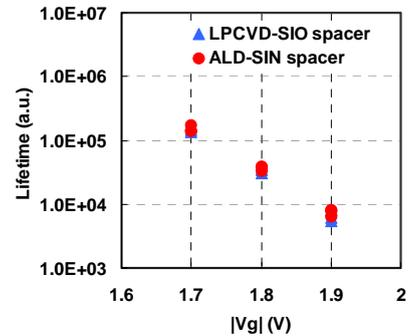
Fig. 12 NBTI of 34 nm gate length of PMOS for ALD-SiN and LPCVD-SiO spacer
