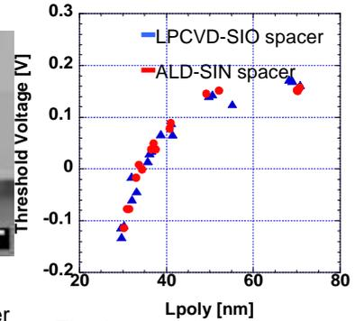
Fig. 4  $V_{th}$ -roll-off characteristics of NMOS
