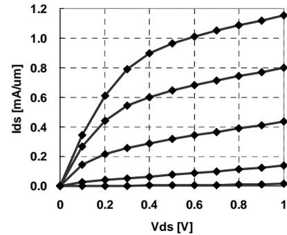
Fig. 5  $I_{ds}$ - $V_{ds}$  characteristics of 34 nm gate length NMOS
