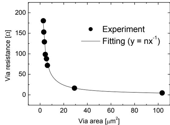
Fig. 5 Via resistance as a function of via area. A solid curve indicates the theoretical calculation.
