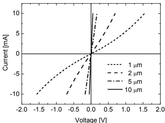
Fig. 4 Typical current-voltage characteristics of planarized CNT vias with various diameters.
