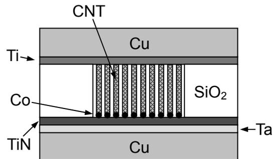
Fig. 1 Schematic diagram of planarized CNT via.
