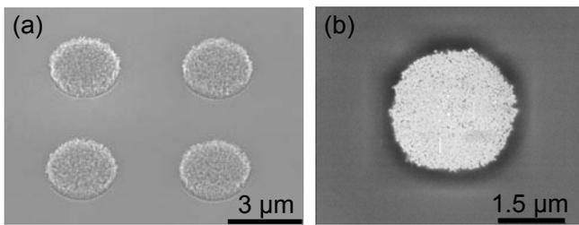
Fig. 3 SEM images of (a) multi-walled CNT bundles grown in via holes and (b) planarized CNT via after CMP.
