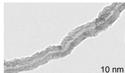
Fig. 2 TEM image of CNT grown by remote plasma-enhanced CVD at 430 °C.
