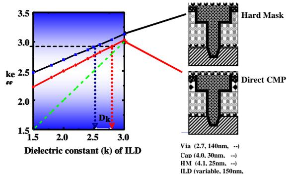
Figure 2 Effective k-values in Hard Mask Retention and Direct CMP Schemes [8]
