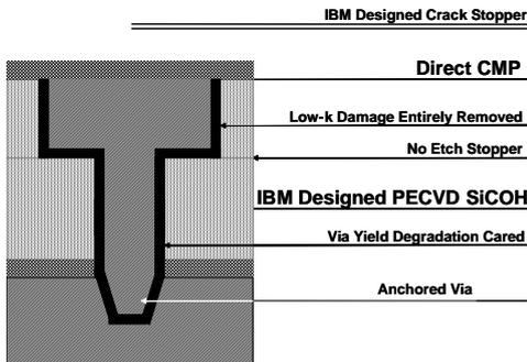
Figure 1 IBM's Monolithic SiCOH Low-k/Cu Integration
