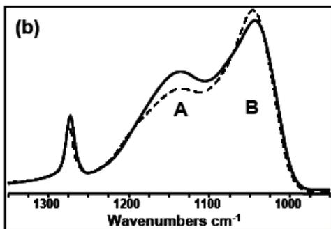
Figure 4 FT-IR spectra of as deposited (solid) and UV cured (dashed) IBM porous SiCOH films [10]
