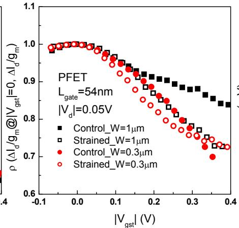
**Fig. 2** Correlation ( $\rho$ ) between  $(\Delta I_d)/g_m$  at  $V_{gst}=0$  and  $(\Delta I_d)/g_m$  at other  $V_{gst}$  vs.  $|V_{gst}|$ . The high correlation coefficient ensures the relevance of the threshold voltage mismatch ( $\Delta V_t$ ) to the drain current mismatch ( $\Delta I_d/I_d$ ).
