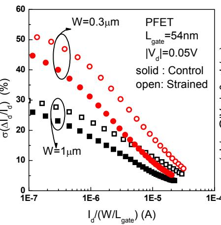
**Fig. 7**  $\sigma(\Delta I_d)/I_d$  vs. normalized  $I_d$  shows larger drain current mismatch for the strained device.
