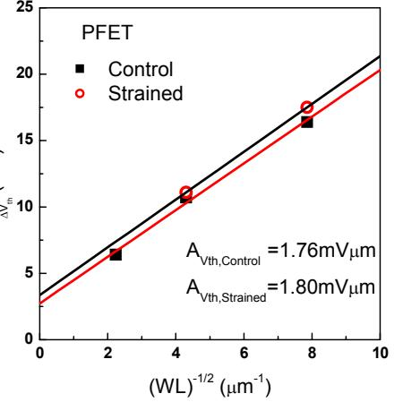
**Fig. 3**  $\sigma(\Delta V_t)$  vs.  $(WL_{gate})^{-0.5}$  shows similar area dependence of  $\sigma(\Delta V_t)$  for the strained and control device.
