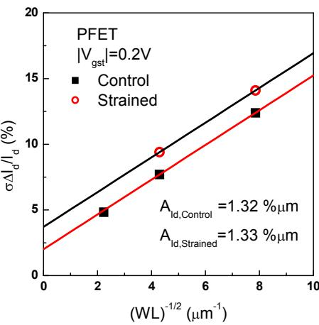
**Fig. 4**  $\sigma(\Delta I_d)/I_d$  vs.  $(WL_{gate})^{-0.5}$  shows similar area dependence of  $\sigma(\Delta I_d)/I_d$  for the strained and control device.
