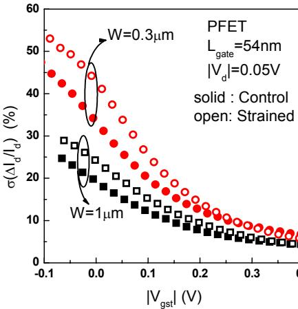
**Fig. 1**  $\sigma(\Delta I_d)/I_d$  vs.  $|V_{gst}|$  shows larger drain current mismatch for the strained device.
