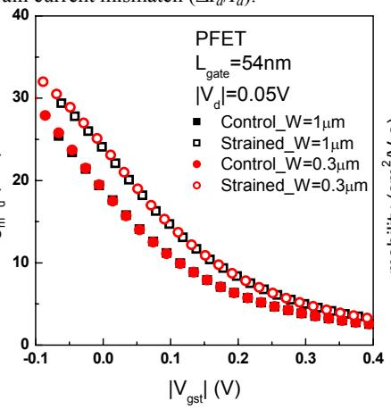
**Fig. 5**  $g_m/I_d$  vs.  $|V_{gst}|$  showing the strain-enhanced  $g_m/I_d$  in the low  $V_{gst}$  region.
