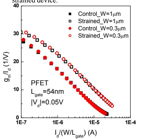
**Fig. 9**  $g_m/I_d$  vs. normalized  $I_d$  showing the strain-enhanced  $g_m/I_d$ .
