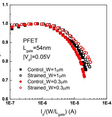
**Fig. 8** Correlation ( $\rho$ ) between  $(\Delta I_d)/g_m$  at  $V_{gst}=0$  and  $(\Delta I_d)/g_m$  at other  $V_{gst}$  vs. normalized  $I_d$ .
