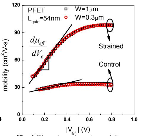
**Fig. 6** The extracted carrier mobility vs.  $|V_{gst}|$  shows larger  $V_g$  sensitivity of carrier mobility in the low  $V_{gst}$  region for the strained device.
