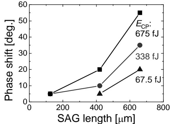
Fig. 5 Dependence of phase shift value obtained from SP on SAG length and excitation energy.
