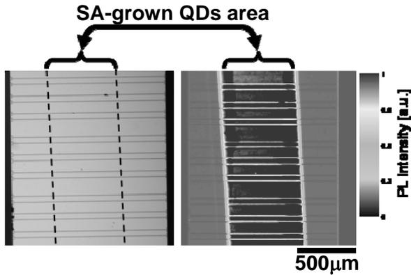
Fig. 3 (a) Optical microscope image of a sample with PC/QD WGs. (b) PL intensity mapping from the sample. High PL intensity of  $1.29\mu\text{m}$  in wavelength obtained from SA-grown QDs clearly demonstrates successful SAG.
