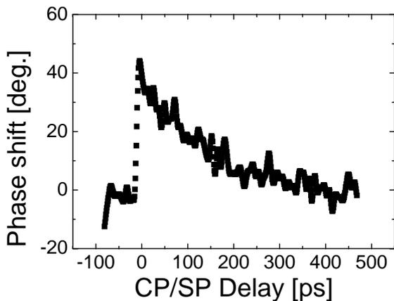
Fig. 4 ONL-induced phase shift of SP against time delay between CP and SP.
