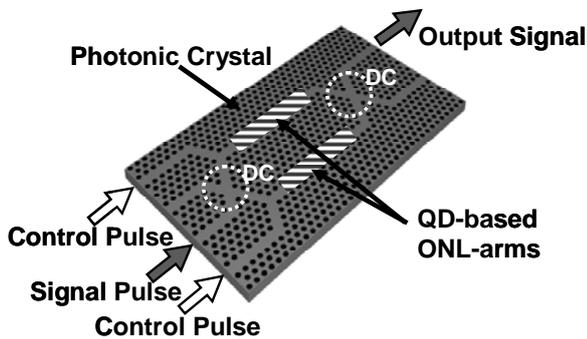
Fig. 1 All-optical switch device, PC-SMZ, composed of PC-WGs and QDs embedded in the ONL-arms. The QDs, which act as a phase-shifter of signal pulses, are preferred to be limited in the ONL-arms.
