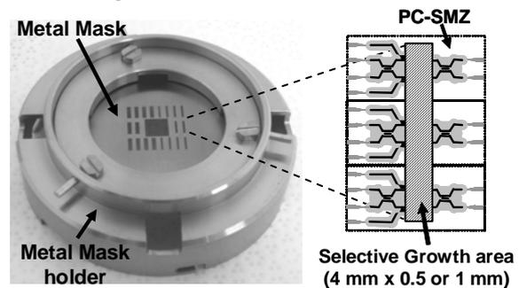
Fig. 2 Metal-mask for the SAG of QDs. Windows pattern on the mask is designed for fabricating PC-SMZ.
