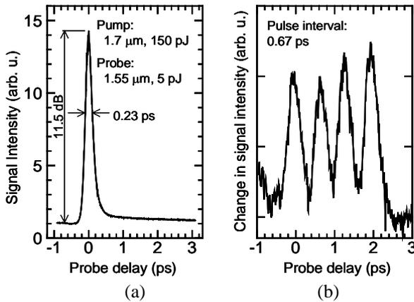
Fig. 2 (a) A gate switch operation with extinction ratio of 11.5 dB and gate width of 0.23 ps. (b) Response for signal pulse trains with an interval of 0.67 ps.
