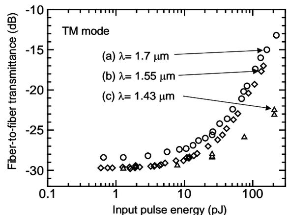
Fig.1 Characteristics of absorption saturation.
