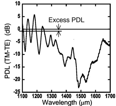
Fig. 3 PDL for a sample grown with carefully optimized growth conditions. The excess PDL is as low as 1 dB.
