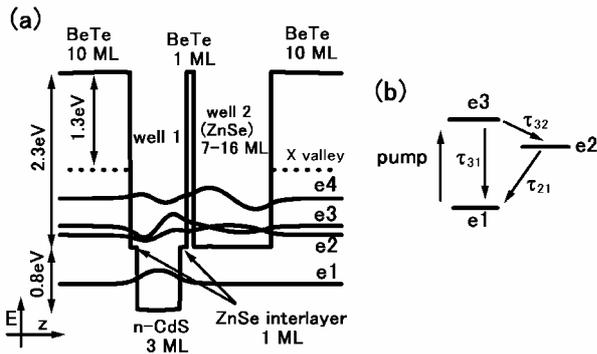
Fig. 1. (a) A representative self-consistent subband structure of II-VI-based CQW with layer parameters, and (b) its intersubband dynamic scheme. e1~e4 denotes the lowest electron states and  $\tau_{ij}$  is the scattering time from  $j$ -th to  $i$ -th subband.
