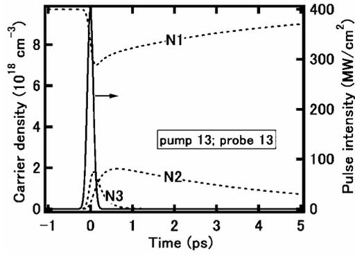
Fig. 3. Response of carrier density at each sublevel under pulse pump. (ij means from  $i$  to  $j$  subbands)
