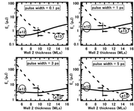
Fig. 6. Structural dependence of  $E_s$  for different pump pulse widths. A dot line with two arrows indicates the dominant intersubband transition.
