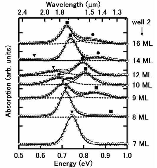
Fig. 2. Intersubband absorption spectra (circles) with different well 2 thicknesses and the corresponding fitting spectra (the solid lines denote the sum of the fitting components (dotted lines)). The markers ( $\nabla, \blacksquare, \bullet$ ) respectively indicate the  $e_{12}$ ,  $e_{13}$  and  $e_{14}$  transitions.
