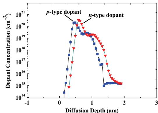
FIG. 2. The *p*- and *n*-type SOD dopant profiles determined using the spreading resistance probe (SRP) method.
