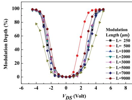
**FIG. 4.** The resultant modulation depths of modulators biased at a constant gate current of 5 mA. The dimensions of the modulators involved in this study all have the width of 7  $\mu\text{m}$  but with different modulation lengths spanning from 250 to 9000  $\mu\text{m}$ .
