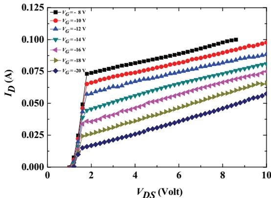
**FIG. 3.** The drain current ( $I_D$ ) versus drain-source voltage ( $V_{DS}$ ) characteristics obtained for a modulator with 11- $\mu\text{m}$ -wide and 2000- $\mu\text{m}$ -long biased with different gate voltages ( $V_G$ ) running from  $-8 \text{ V}$  to  $-20 \text{ V}$  at an increment of  $-2 \text{ V}$ .
