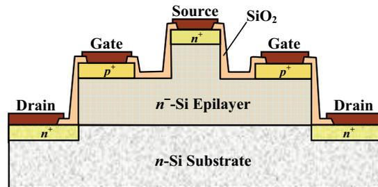
FIG. 1. A schematic diagram of a silicon modulator based on the three-terminal transistor waveguide structure.
