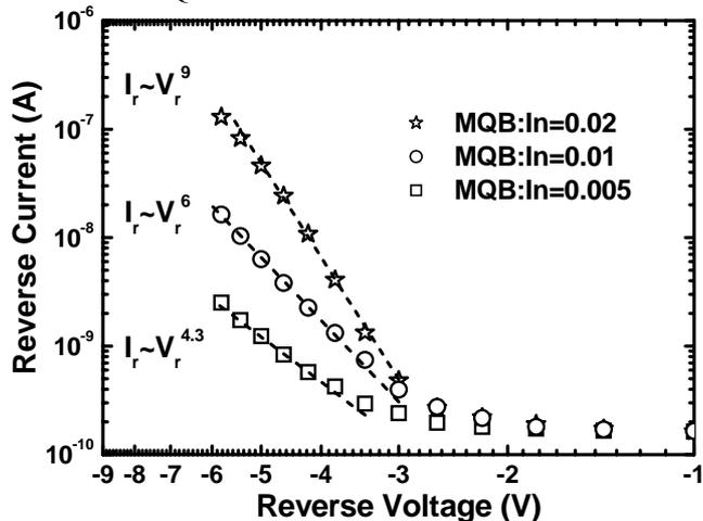
Fig.2. Reverse current vs voltage on a log-log scale for the LEDs with MQBs. The In compositions of the MQBs for these samples were 0.005, 0.01, and 0.02, respectively.
