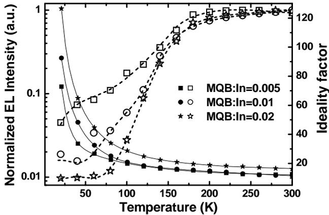
Fig. 1. Normalized EL intensity and ideality factor as a function of temperature for the LEDs with MQBs. The In compositions of the MQBs for these samples were 0.005, 0.01, and 0.02, respectively.
