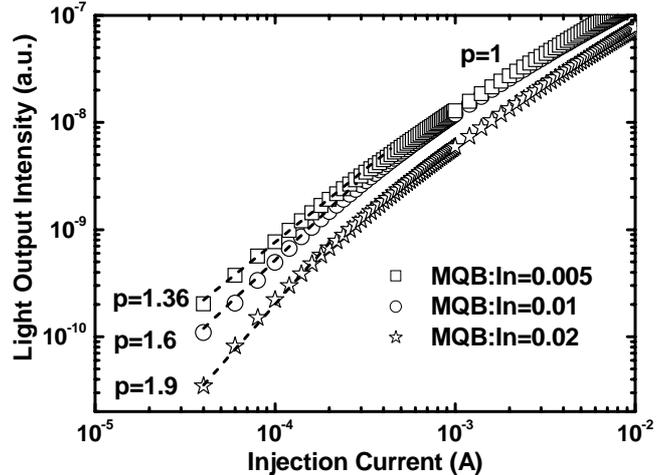
Fig. 3. Dependence of light output on the injection current for the LEDs with MQBs. The In compositions of the MQBs for these samples were 0.005, 0.01, and 0.02, respectively.
