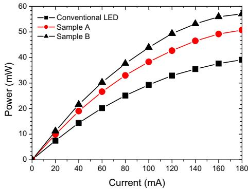
Fig. 3. Output power of sample A, sample B, and conventional LEDs measured by an integral-sphere as a function of a forward dc current.
