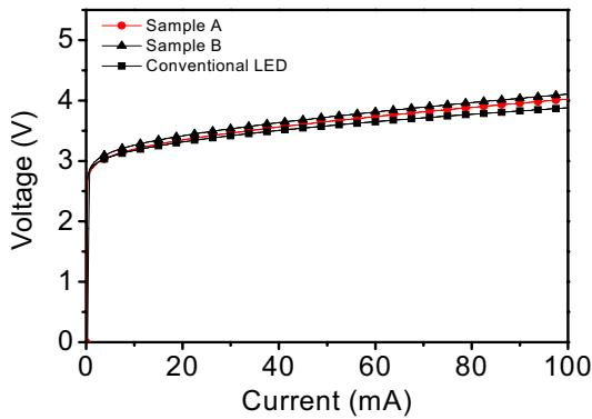
Fig. 2. The  $I$ - $V$  forward curve of sample A, sample B and conventional LEDs fabricated in this investigation.
