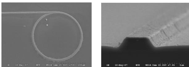
Figure 3. SEM pictures of the etched ridge waveguide structure by excimer laser assisted chlorine etching at 140 K.
