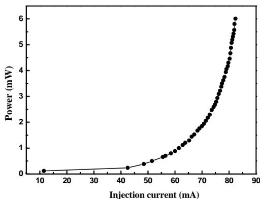
Figure. 4 L-I curve of the fabricated circular ring laser, the threshold current is around  $70\ \text{mA}$ .
