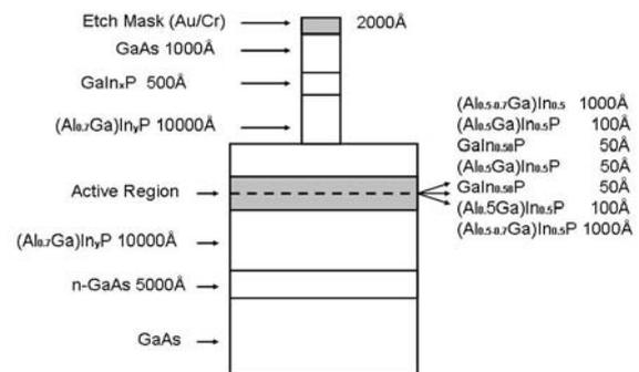
Figure. 1 The MOCVD grown InGaAlP multiple quantum wells structure.
