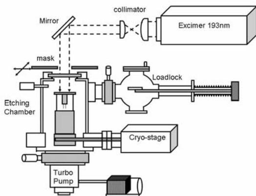
Figure 2. The sketch of the excimer laser assisted cryo-etching system
