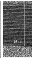
Fig6: TEM view of twin HSQ pattern on both side of Si layer.
