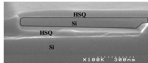
Fig4:Conformity of HSQ deposition in cavities.
