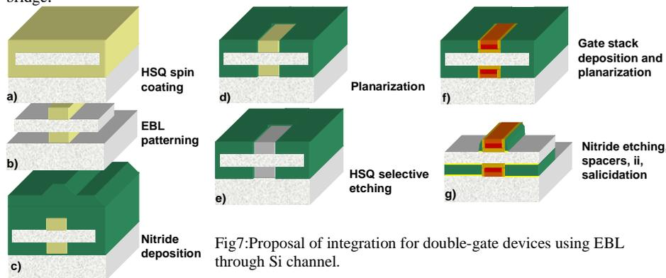
Fig7:Proposal of integration for double-gate devices using EBL through Si channel.
