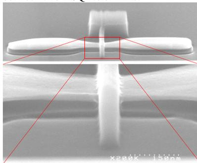
Fig5:HSQ dummy gate around silicon bridge.
