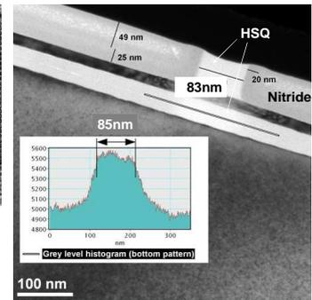
Fig8: TEM view of nitride planarization step (fig7d)
