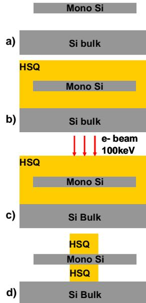
Fig2: Sequence of Electron Beam lithography through thin Si layer.
