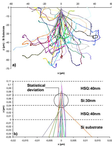
Fig1 : Monte Carlo simulation of electron trajectories @100keV a) in substrate b) through Si layer between two HSQ resist films.
