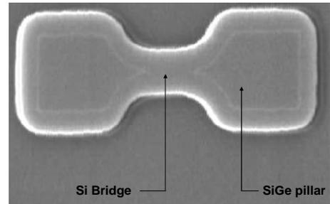
Fig 3: High Energy SEM top view of a silicon layer hanging up by SiGe pillars.
