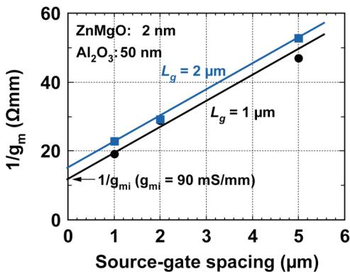
Fig. 3 Reciprocal transconductance  $1/g_m$  vs. source-gate spacing for  $\text{Al}_2\text{O}_3$  gate devices.
