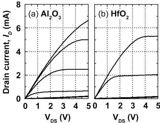
Fig. 2  $I_D$ - $V_{DS}$  characteristics of 1- $\mu\text{m}$ -long gate devices for gate dielectrics of  $\text{Al}_2\text{O}_3$  (a) and  $\text{HfO}_2$  (b), respectively. A larger transconductance was observed for the  $\text{HfO}_2$  gate dielectric.
