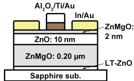
Fig. 1 Cross-sectional structure of a ZnO/ZnMgO hetero-MIS FET.
