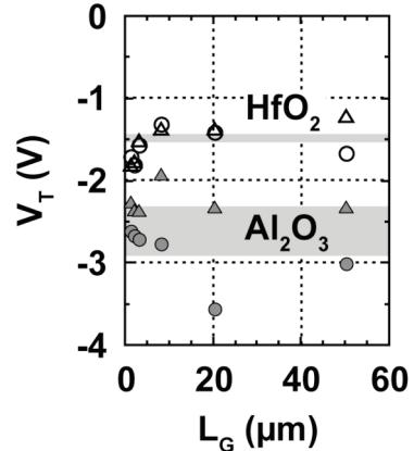
Fig. 4 Hysteresis characteristics for the gate dielectrics of  $\text{Al}_2\text{O}_3$  and  $\text{HfO}_2$ .
