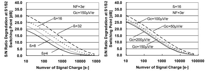
Fig.4 SNR degradation simulation at signal switching point.
