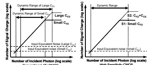
Fig.2 The high sensitivity solution overcoming the dynamic range trade-off compared with the conventional approach.
