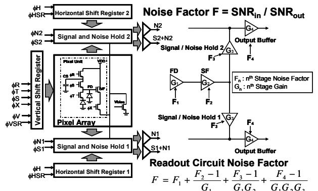
Fig.1 The sensor block diagram and the formula of noise factor.
