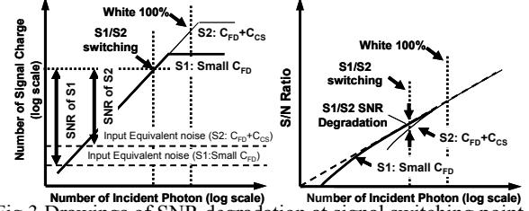
Fig.3 Drawings of SNR degradation at signal switching point.
