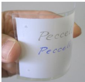
Fig. 1 TiO 2 -coated ITO-PEN film for dye-sensitized plastic photo-electrode showing high hardness against writing by pencil (upper) and ball-point pen (lower).
