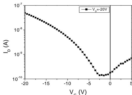
Fig. 3  $I_D$ - $V_G$  transfer characteristics of printed OTFT(collaboration with J.B. Koo, ETRI)
