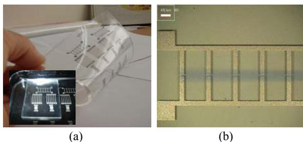
Fig. 2 Results of OTFT fabrication in: (a) 5'' size h-PDMS stamp with channel lengths of 5 $\mu$ m, 10 $\mu$ m, and 20 $\mu$ m(width=500 $\mu$ m), (b) printed source/drain electrodes on ITO and parylene formed PEN substrate using conductive Ag ink, and ink jetting semiconductor
