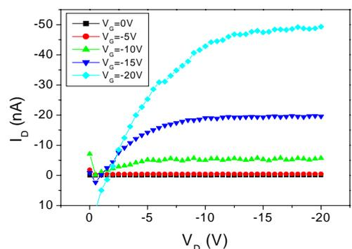
Fig. 4  $I_D$ - $V_D$  output characteristics of printed OTFT(collaboration with J.B. Koo, ETRI)
