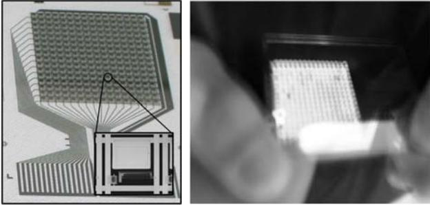
Figure 3. Images of fabricated printed OTFT-OLED array
