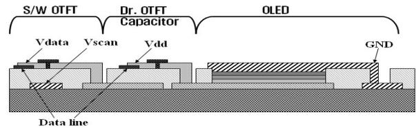
Figure 1. The cross section of pixel
