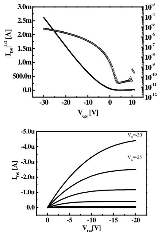
Figure 2. The electrical characteristics of printed OTFT
