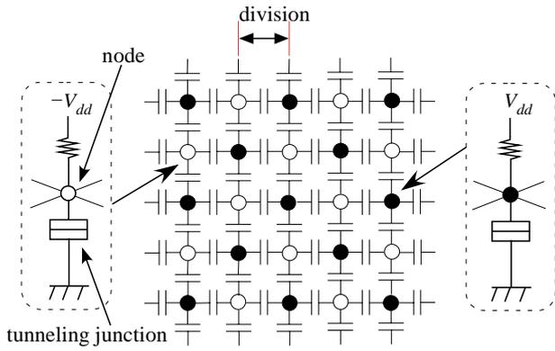
Fig. 1 Photon position sensor consisting of a network of single-electron oscillators. Closed circles and open circles are the nodes of positively and negatively biased oscillators respectively.
