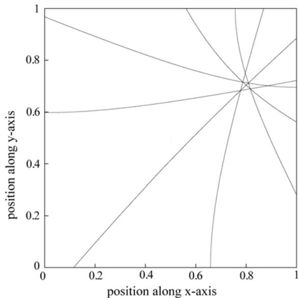
Fig. 5 Calculation of the starting position of tunneling waves. The six hyperbolas with their 15 intersection points are shown. The mean coordinate of the intersection points was  $(0.799, 0.701)$  and approximately consistent with the actual starting position  $(0.8, 0.7)$ .
