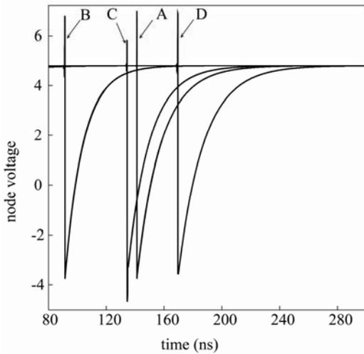
Fig. 3 Node voltage wave forms of the oscillators at corners A, B, C, and D of the device.
