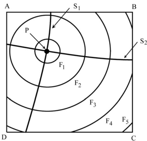
Fig. 4 Determination of the position of incident photons, making use of wave propagation. ABCD: device surrounded by a square periphery. P: incident position of a photon, or the starting point of a tunneling wave. F1-F5: spreading wave front for four time steps. S1 and S2: two hyperbolas given by arrival-time data for points A,B, and C.
