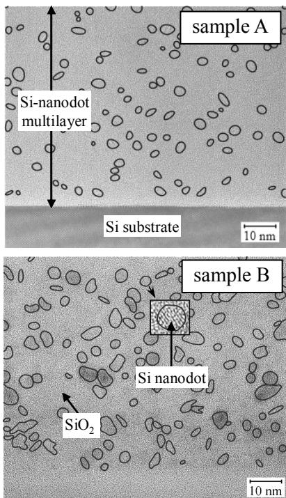
**Fig. 1.** Cross-sectional TEM images for Si-nanodot multilayers with oxidation temperature of 800 °C (sample A) and 600 °C (sample B).
