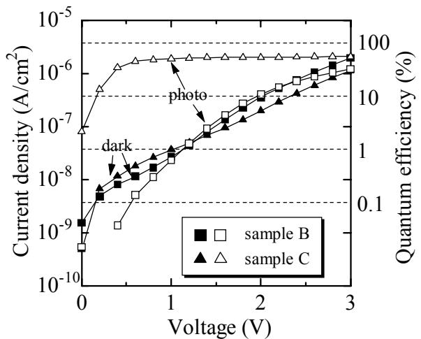
**Fig. 5.** Current-voltage characteristics for sample B and C under illumination by 4.1 eV monochromic light.
