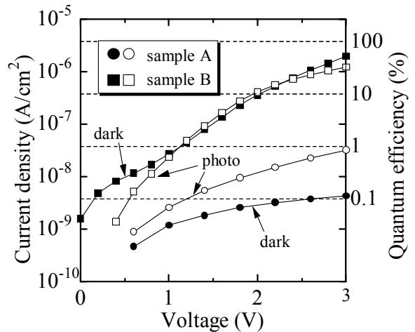
**Fig. 3.** Current-voltage characteristics for sample A and B under illumination by 4.1 eV monochromic light.
