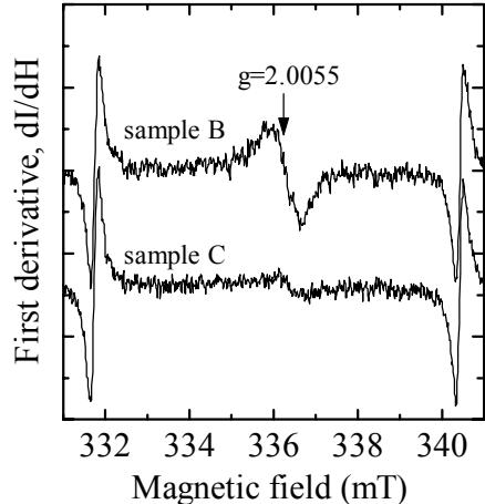
**Fig. 4.** ESR spectra before atomic hydrogen annealing (sample B) and after atomic hydrogen annealing (sample C).
