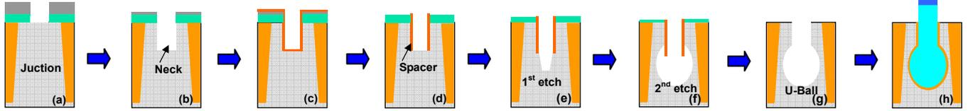
Fig.2 Core process flow of U-RCAT structure. The two step etching processes with different etching rates plays an important role in the formation of the U-RCAT structure. The U-RCAT realizes better performance and reliability with the same area as the S-RCAT, which illustrates the powerful scale-down ability of the U-RCAT versus S-RCAT.
