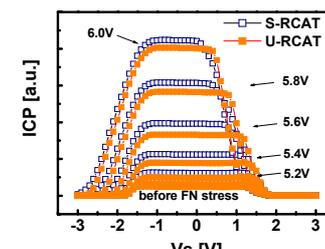
Fig. 14 The ICP distributions with FN stress are improved in U-RCAT due to less leakage current and smooth neck curvature. (FN stress for 60s)
