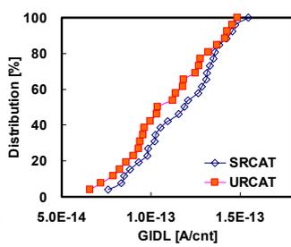
Fig. 10 GIDL currents of the U-RCAT are reduced, which helps increase data retention time.
