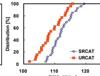
Fig. 7 SW Distribution of U-RCAT is improved due to the flatter ball bottom channel and  $E$ -field relaxation.
