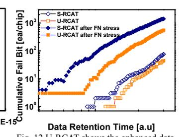
Fig. 12 U-RCAT shows the enhanced data retention time due to the improved GIDL, junction leakage current, and the  $E$ -field relaxation. ( $t_{RC}=10\text{min}$ )
