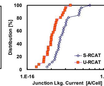
Fig. 11 Junction leakage current of the U-RCAT is improved due to less junction area.
