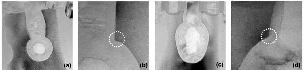
Fig. 4 TEM images of (a) S-RCAT, (b) neck of S-RCAT, (c) U-RCAT, and (d) neck of U-RCAT. The neck curvature of U-RCAT increases by  $120\sim 130^\circ$  compared with  $100\sim 110^\circ$  in the S-RCAT. U-RCAT shows the smoother and wider neck curvature.
