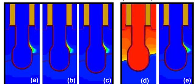
Fig. 15 Device simulation profiles of U-RCAT with ball depth of (a)  $100\text{\AA}$ , (b) target, (c)  $100\text{\AA}$ , (d)-(e) the optimal U-RCAT, which shows the least  $E$ -field. The  $E$ -field is negligible with the U-ball depth, but the data retention time is very sensitive with the U-ball depth and diameter.
