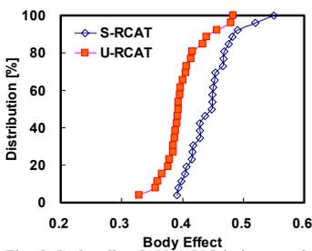
Fig. 9 Body effect  $[\Delta V_{th}/\Delta V_b]$  is improved in the U-RCAT due to greater width.
