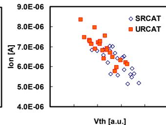
Fig. 6 Correlation curves between the  $I_{on}$  and  $V_{th}$ . The Ion of U-RCAT are enhanced by improving SW and DIBL.
