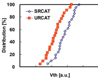
Fig. 5 The  $V_{th}$  of the U-RCAT decreased due to the improved SW.
