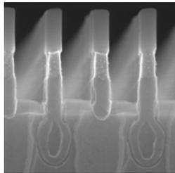
Fig. 3 Vertical SEM image of U-RCAT after forming gate.
