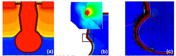
Fig 1. Simulation profiles of S-RCAT structure. It is shown that  $E$ -field intensity is highly concentrated in the neck curvature due to the stiff neck angle of  $100\sim 110^\circ$ .
