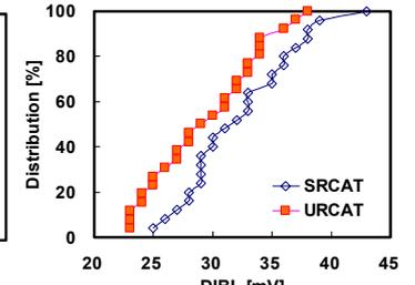
Fig. 8 DIBL distribution of the U-RCAT shows better properties than that of S-RCAT due to the increased  $L_{eff}$ .
