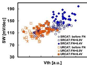
Fig. 13 U-RCAT shows the enhanced FN stress immunities due to the relaxed  $E$ -field at the neck curvature and a better SW.
