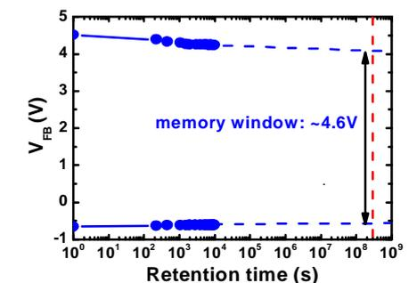
Fig. 12 Retention characteristic of nanocrystal memory devices. A large memory window is observed after 10 years of retention.
