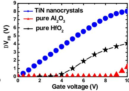
Fig. 5  $V_{FB}$  shift as a function of positive gate voltage. The TiN nanocrystal shows large  $V_{FB}$  shift, while the pure Al<sub>2</sub>O<sub>3</sub> does not show any hysteresis memory window up to gate voltage of 9 V.
