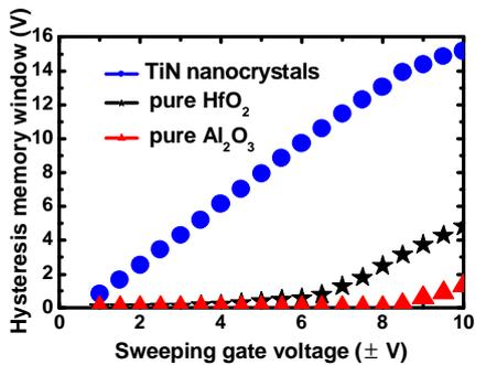
Fig. 7 Hysteresis memory window versus sweeping gate voltage for all memory devices.
