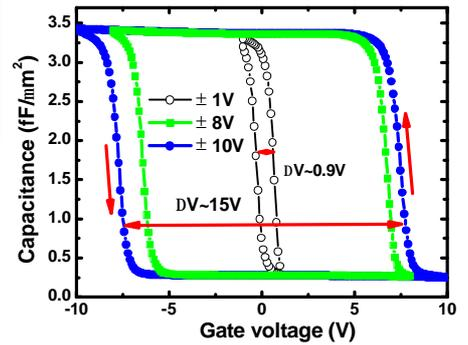
Fig. 3 The C-V (1 MHz) hysteresis shows a large memory window of ~15V@ V<sub>g</sub> = ±10 V. The hold time was 100 ms during C-V measurement.
