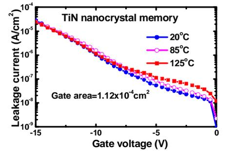
Fig. 9 A negligible leakage current increases with increasing measurement temperature, due to the Al<sub>2</sub>O<sub>3</sub> blocking oxide and Pt gate.
