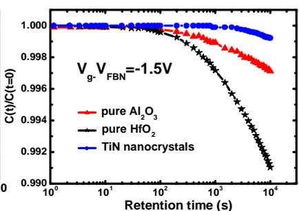
Fig. 11 Discharge characteristics of nanocrystal memory devices. Discharges are studied after  $V_g - V_{FBN} = 6V$ , 10s stressed condition. The  $V_{FBN}$  is the  $V_{FB}$  at neutral C-V (no hysteresis memory window).
