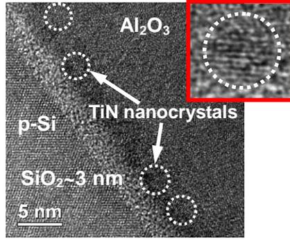
Fig. 2 Cross-sectional HRTEM image of atomic layer deposited TiN nanocrystals after 900°C, 2 min process. The diameter of TiN nanocrystal is less than 3 nm (in the inset).
