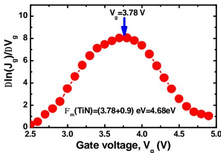
Fig. 4 Current density ( $J_g$ ) versus gate voltage ( $V_g$ ) characteristics is measured using Si/Al<sub>2</sub>O<sub>3</sub> (8 nm)/TiN structure. The calculation of work function ( $\Phi_m$ ) for TiN metal layers has been explained in the ref. [8].
