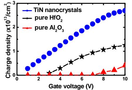
Fig. 6 Charge density as a function of positive gate voltage. The pure Al<sub>2</sub>O<sub>3</sub> has negligible charge trapping density as compared with nanocrystal memory capacitors.
