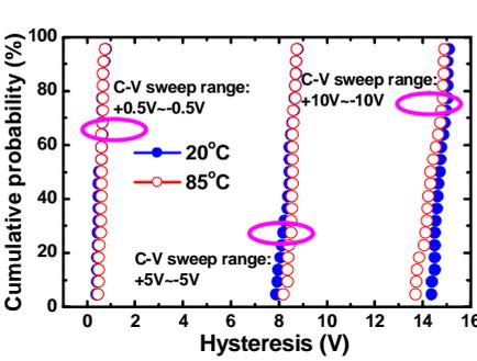
Fig. 8 Cumulative probability of C-V hysteresis of TiN nanocrystal memory capacitors.
