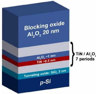
Fig. 1 Memory structure of ALD TiN (0.5 nm)/Al<sub>2</sub>O<sub>3</sub> (1 nm) multilayers on SiO<sub>2</sub> (3 nm)/p-Si substrate. The thickness of Al<sub>2</sub>O<sub>3</sub> blocking oxide was 20 nm.
