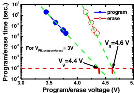
Fig. 10 Program/erase characteristics with high work function metal gate (Pt). The TiN nanocrystal memory device can be used for very low power applications.
