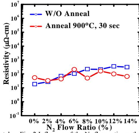
Fig. 2 Influence of the  $N_2$  flow ratio on the resistivity of the  $Hf_xMo_yN_z$  films deposited on the silicon oxide.
