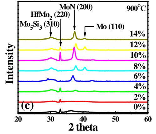
Fig. 4 XRD patterns of the  $Hf_xMo_yN_z$  films with various  $N_2$  flow ratio. (a)W/O anneal (b) Anneal 700°C, 30 sec (c)Anneal 900°C, 30 sec.
