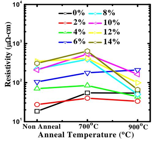
Fig. 3 The annealing temperature effects on resistivity of  $Hf_xMo_yN_z$  thin films were relative.
