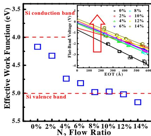
Fig. 7 Work function of  $Hf_xMo_yN_z$  as a function of the  $N_2$  flow ratio ( $\Phi_{m,eff} = 4.17\text{eV} \sim 5.16\text{eV}$ ).
