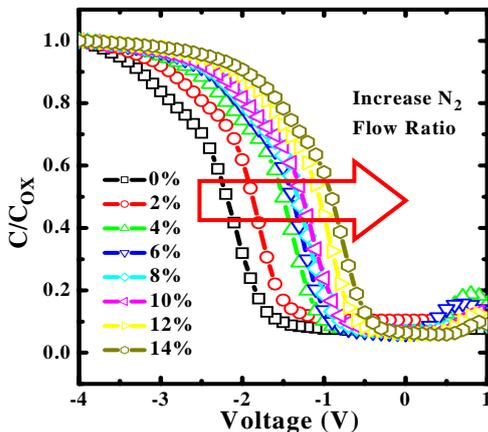
Fig. 6 Normalized C-V curves of  $Hf_xMo_yN_z$  gates with various  $N_2$  flow ratio on  $SiO_2/p$ -type Si.
