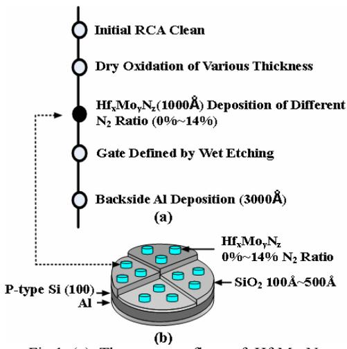
Fig.1 (a) The process flow of  $Hf_xMo_yN_z$  metal gate MOS capacitors. (b) Schematic cross-section for  $Hf_xMo_yN_z$  metal gate MOS capacitors in this work.
