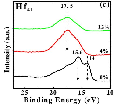
Fig. 5 XPS spectra of the  $Hf_xMo_yN_z$  thin films with various  $N_2$  flow ratio. (a): N(1s), (b): Mo(3d), (c): Hf(4f).
