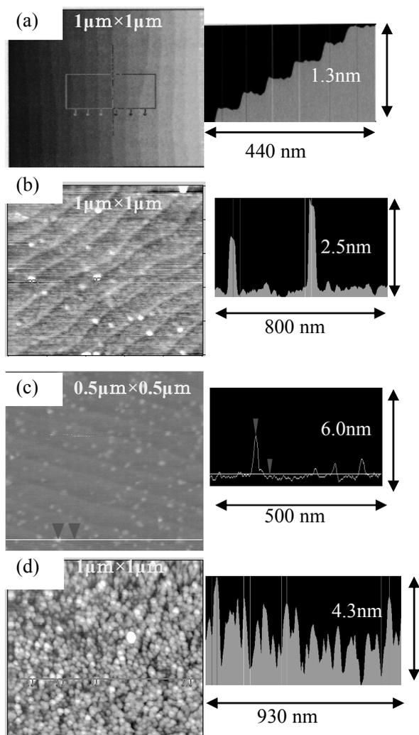
Fig. 1 DFM images and height profiles of the sapphire surfaces. (a) Single-stepped sapphire surface. (b) and (c) Avidin-terminated single-stepped surfaces where avidin densities in the solutions were 20 nM and 160 nM, respectively. (d) Avidin-terminated randomly-stepped surfaces where avidin density in the solution was 20 nM.
