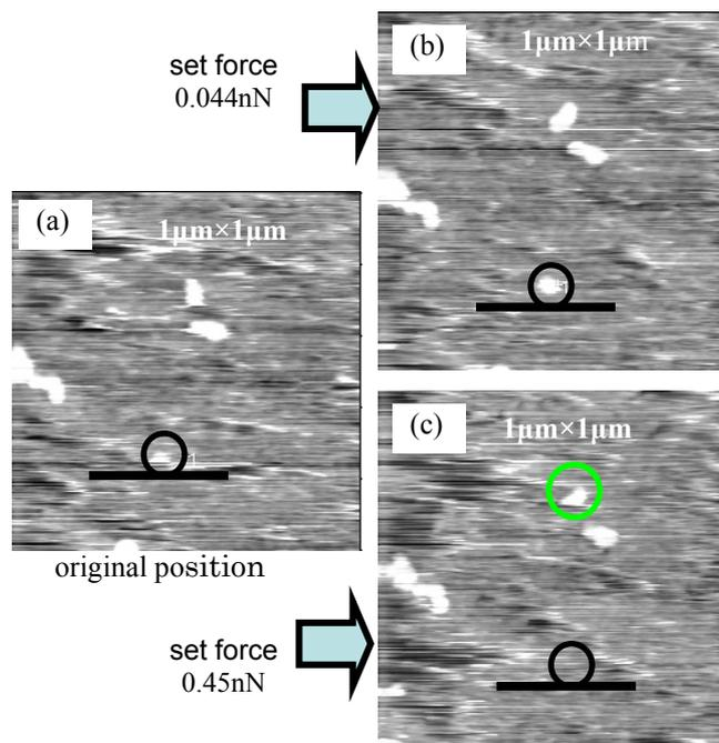
Fig. 2. DFM images of the sapphire surfaces (a) before the scan of the frictional force mode, (b) after the scan with the set force of 0.044 nN, and (c) after the scan with the set force of 0.45 nN.
