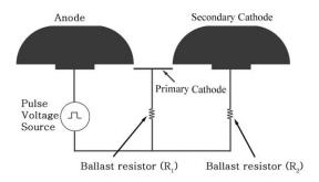
Fig. 2 Schematic of test setup for plasma generation.
