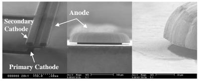
Fig. 1 SEM images of fabricated micro triode.
