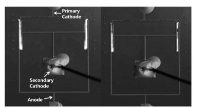
Fig. 4 Photographic images of microplasma operated in glow discharge mode at atmospheric Ar ambient. (a) rise time: 100 ns (b) rise time: 800 ns
