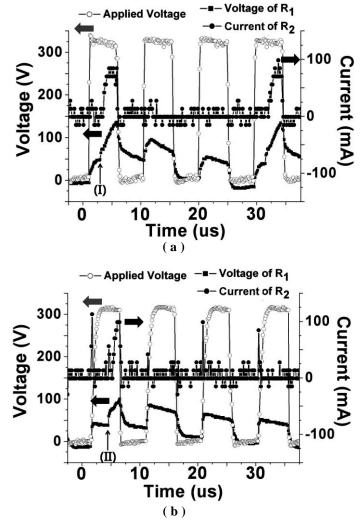
Fig. 5 I-V characteristics of micro triode operated in the glow discharge mode. Arrows point out initiation of gas breakdown, indicted by region (I) and (II). (a) rise time: 100 ns (b) rise time: 800 ns
