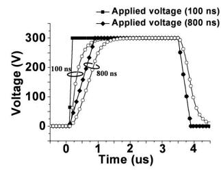
Fig. 6 Simulated voltage delay at microelectrodes prior to gas breakdown using SPICE. Open symbol: induced voltage across electrodes. Note that a RC delay of nearly 1 us between two pulses is caused by capacitance and resistance of microelectrodes.
