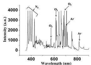
Fig. 3 Emission spectrum of generated microplasma. Argon was used as the carrier gas in ambient air for the discharge experiment.
